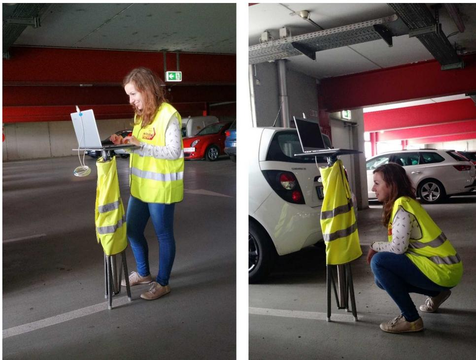
**Figure 7.12:** To avoid obstructing the signal path, the observers knelt down while the RSS were being recorded.
