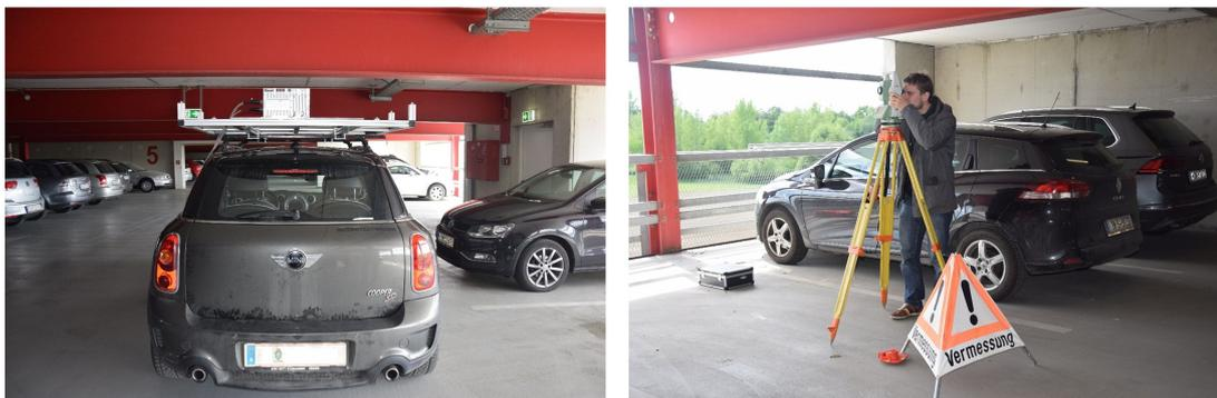
**Figure 7.10:** An IMU and tachymeter measurements are needed to obtain the reference trajectory.
