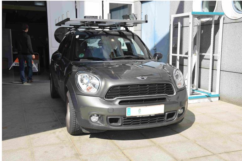
**Figure 7.9:** Test vehicle with the sensor platform mounted on the roof.
