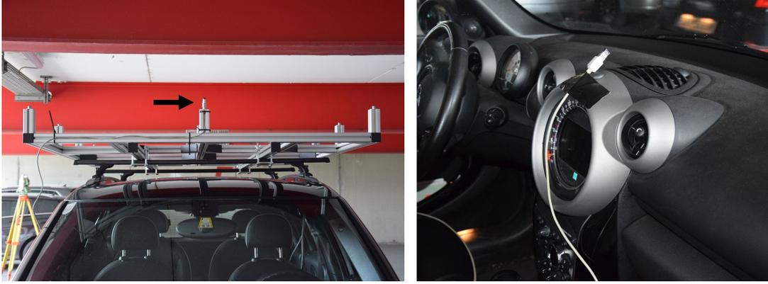
**Figure 7.11:** The BLE antenna was first mounted on the platform (left) and then placed inside the vehicle (right).
