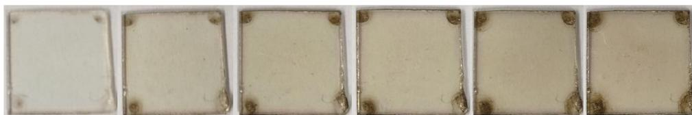
Figure 32: Substrates with increasing number of layers of CIS nanocrystals on  $\text{TiO}_x$  (left to right: 1, 3, 5, 7, 9, 11)
