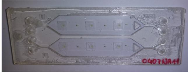
The Finished Sensors in a 250 $\mu$ L Rhombic Chamber Chip. Beginning from the Left there is Alternatively a Glucose Sensor and an Oxygen Sensor Next to Each Other.
