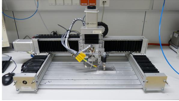
**Figure 4.6:** The Setup of the Computerised Numerical Control and the Microdispenser
