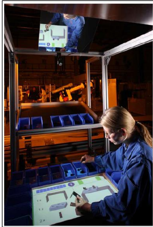
Figure 4: Experimental workplace for displaying assembly instructions, based on a multi-dimensional complexity-measurement (Zaeh, et al., 2009)
