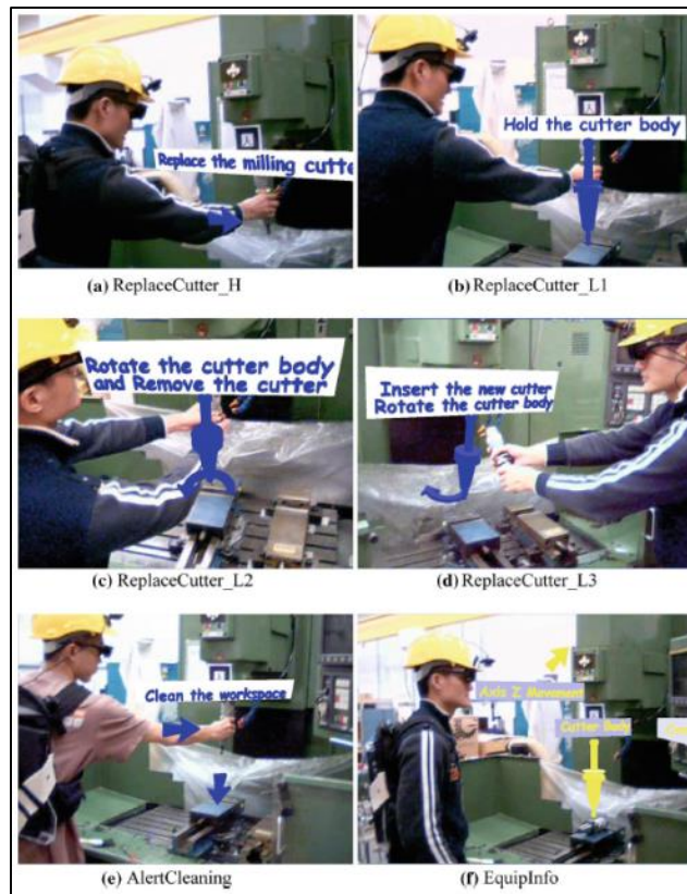
Figure 9: Context aware AR maintenance assistance (Zhu, et al., 2014)
