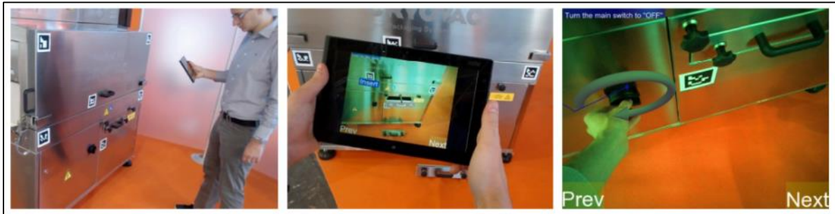
Figure 17: User frames machine with tablet (left) and looks at the instructions by means of the tablet (center and right) (Re & Bordegoni, 2014)
