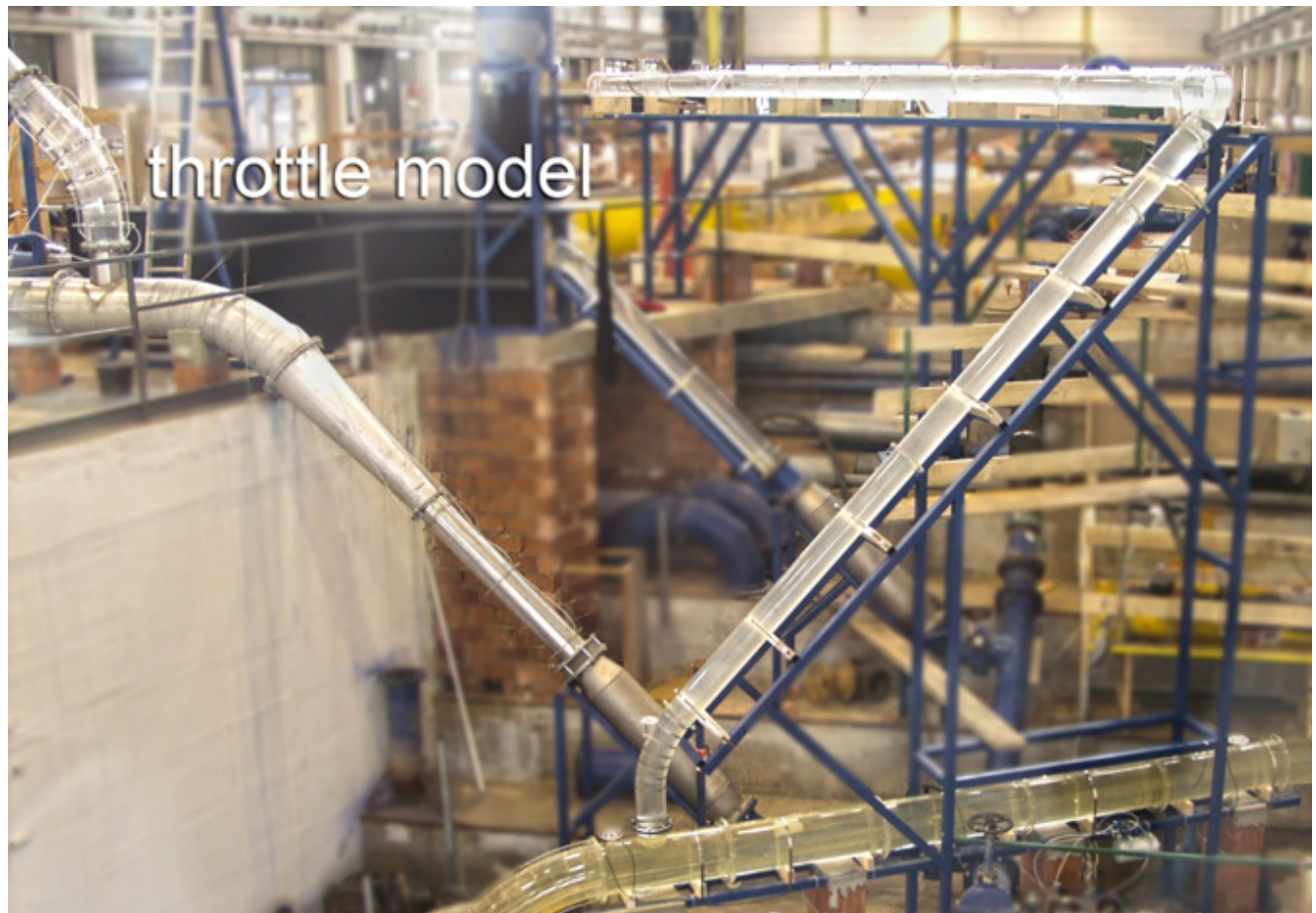
Scale model [M 1:30] of the surge tank of Limberg II at TU Graz
