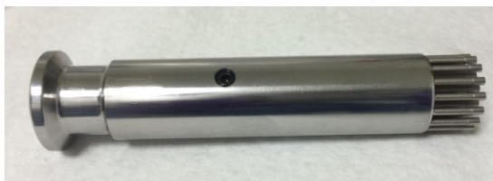
Figure 6: Monoblock punch, 24 tips, side view
