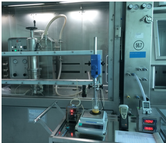
Figure 29: Experimental setup Fluidized bed coating Mini-Glatt
