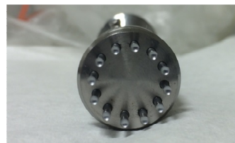
Figure 5: Multiple part assembly punch, 12 tips, frontal view
