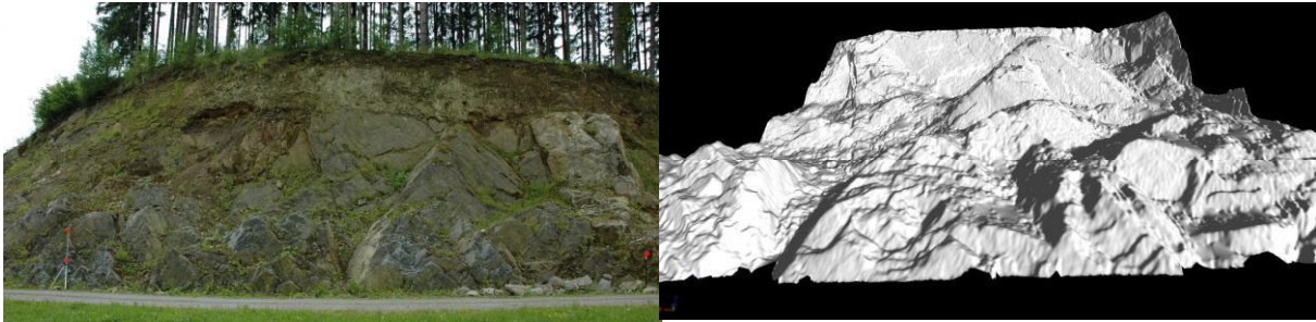
Figure 5: Example of an outcrop and the generated DEM (Liu, 2016).
