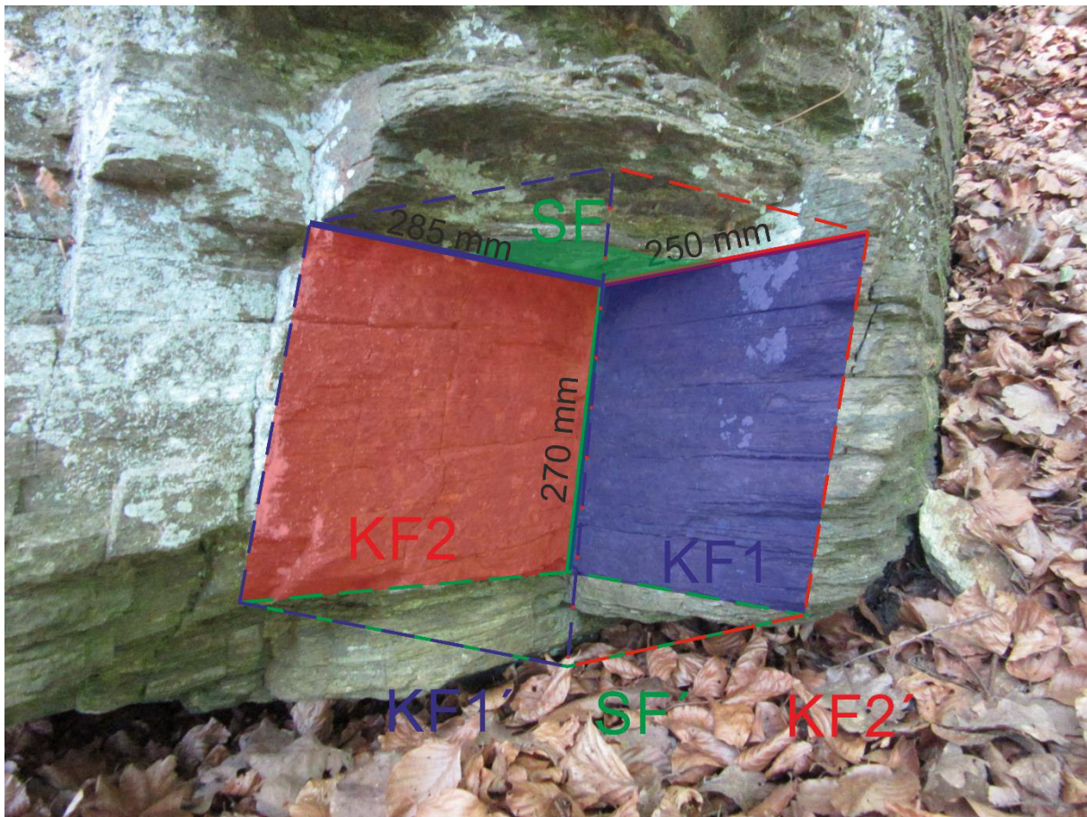
Figure 17: Mould 1 (Marhof, Stainz), showing all joints and free planes.
