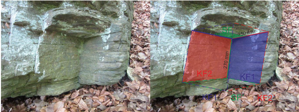
Figure 8: Block mould on a natural rock slope and the governing joint sets KF1 (blue), KF2 (red) and SF (green) which comprise the block.
