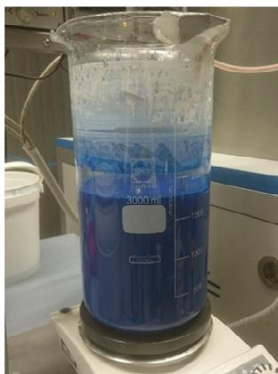
Figure 20: Indigo carmine spraying suspension (2w%)
