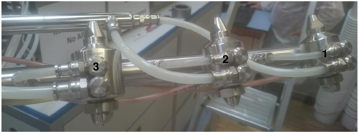
Figure 6: The three spraying nozzles (1-3).
