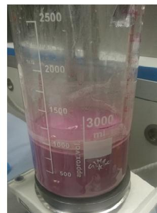
Figure 21: Iron-(III)-oxide spraying suspension (10w%)
