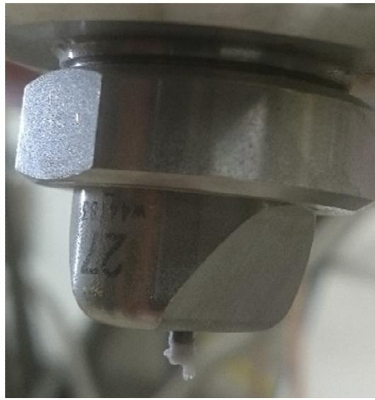
Figure 43: Blocked nozzle.
