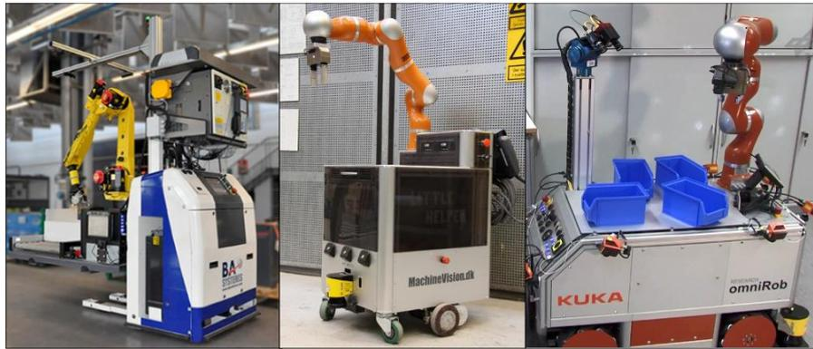
Figure 8: Autonomous industrial mobile manipulators – project STAMINA [3] (left), project TAP-AS [62] (middle) and the project of DLR [40] (right)
