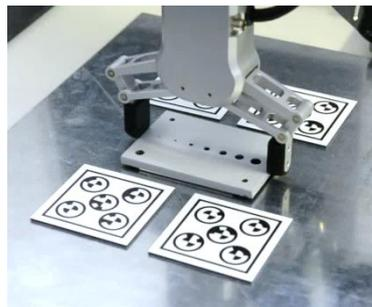
Figure 144: Final pick position of the robot TCP with respect to the object
