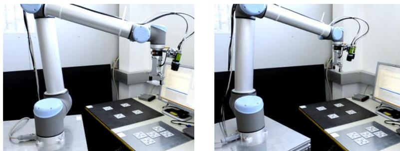
Figure 145: Change of the RCS between the pick and place operation by moving the mobile platform
