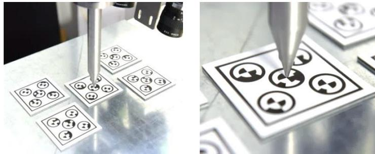
Figure 137: TCP pose of the robot at the extrapolated target pose of the M2M-Map
