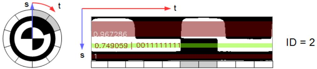
Figure 60: 3D Fiducial Propeller marker – the variation of  $s$  and  $t$  can be used to create a mapping for the  $x$  and  $y$  direction. The remapping of the marker results in a rectangular image that can be used to extract the marker identification (adapted from [56]).
