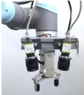
Figure 71: End-effector of the industrial robot with stereo system and gripper
