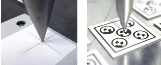
Figure 151: Extrapolated TCP target pose of the M2O-Map (left) and the M2M-Map (right) with the use of 50 support points uniformly distributed between the object Z offset of 450 mm and 150 mm.
