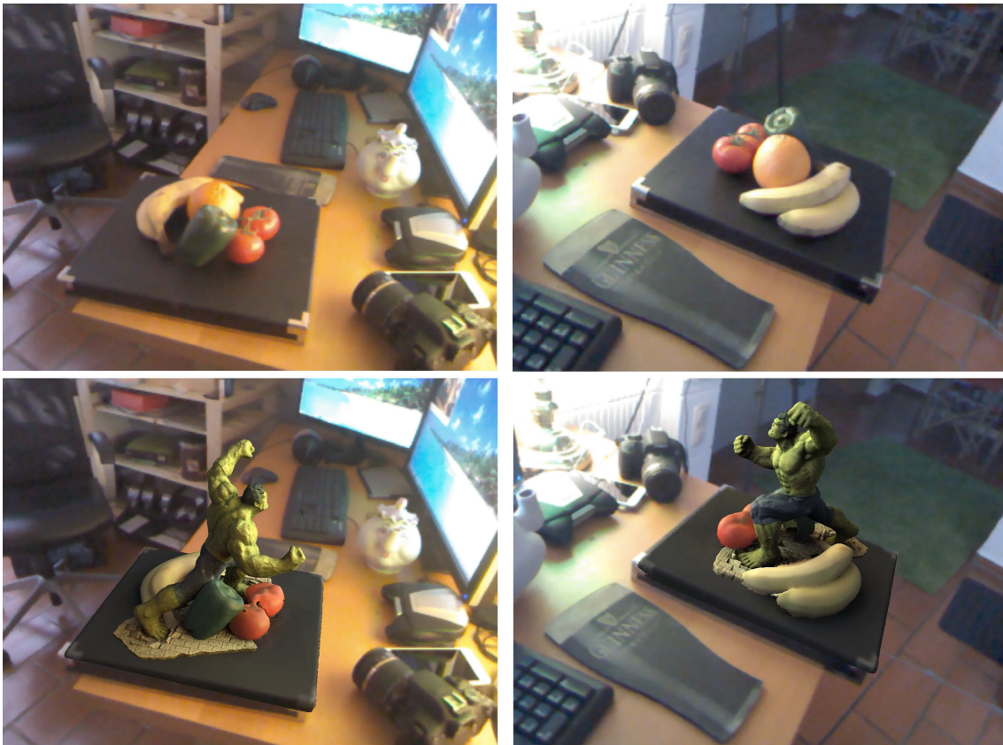
Figure 5.9: Interchanged Augmented Reality. Geometry reconstructed from a real scene shown in Figure 5.8 gets inserted into another real scene matching the lighting. To support inter-reflections like self-shadow the target geometry is rendered in addition.
