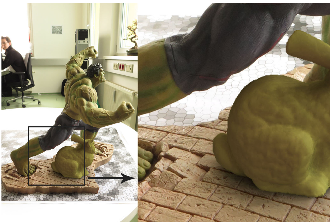
Figure 5.8: Differential Rendering. Image shows strong self shadow effects from recovered geometry to virtual geometry and vice versa.
