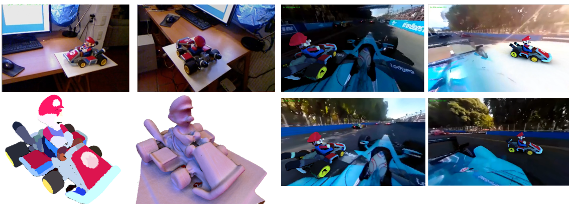
Figure 5.10: Augmented Reality. (left) Input data and estimated albedo color and lighting. (right) We place the scan inside a 360 video and relight the geometry using our material estimated and an estimation of lighting in each video frame video.
