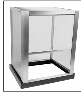
Figure 5.17.: Faraday cage for the whole worktop [29]
