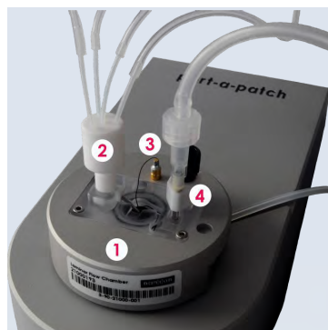
Figure 5.24.: Laminar Flow Chamber; Faraday lid with the chamber (1), including the nozzles (2), the external ground electrode (3), and the waste removal connector (4) [39]
