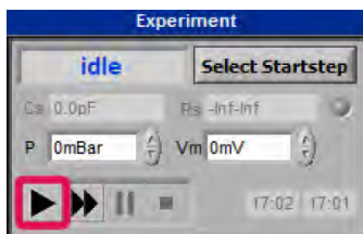
Figure 5.30.: Push the play button in the experiment window to start the measurement [39]
