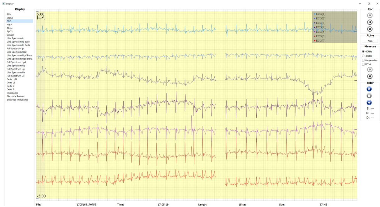
Figure 5.3: SmartNIBP display. On the right side are the controls to switch views and to save and pause the data. [Screenshot taken by the author].
