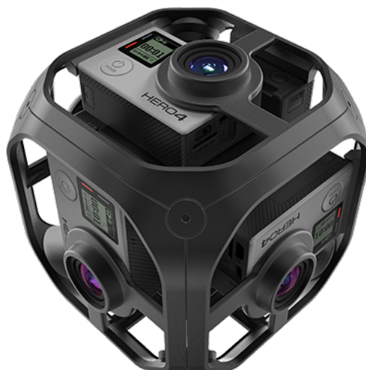
Abbildung 6: GoPro Omni - 360° Rig Quelle: GoPro Inc. http://www.gopro.com/ Zugriff: April 2017
