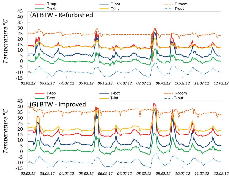
Figure 3-5: Extraction of the Monitored Temperatures in February 2012 for (A) Refurbished and (G) Improved BTWs
