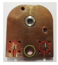
Figure 3.8: A photograph of the copper plate. The red circles mark the places where the TEM grids are mounted and the green circle marks the hole which is used for the deposition on fused silica.
