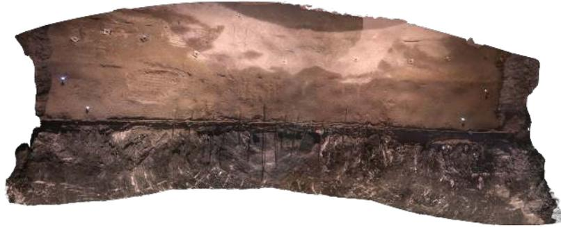
(a) 2D projection of tunnel surface onto a tunnel profile raster (profile arc length vs. tunnel axis direction). Rock excavation surface at bottom, shotcrete protection with anchors and steel arches at top.
