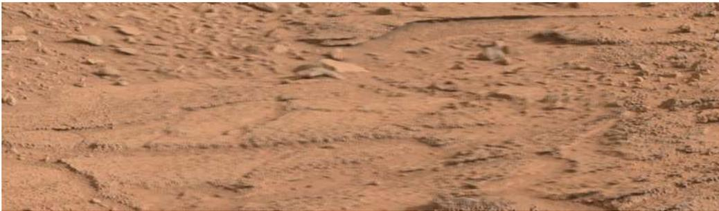
(a) Image detail stitched with raw pointing information. A shift in horizontal direction is clearly visible as blurred area with duplicated structures.
