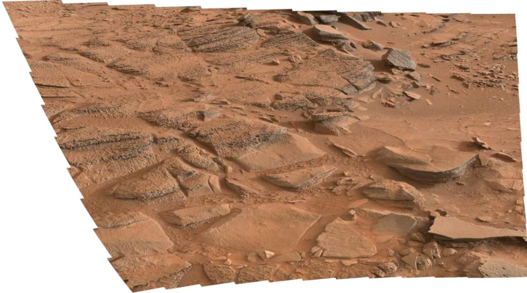
Figure 4.11: JR Warping approach. The resulting image is a seamless panorama with no major artefacts. Radiometric seams are not visible due to blending. Image courtesy by NASA/JPL/JR
