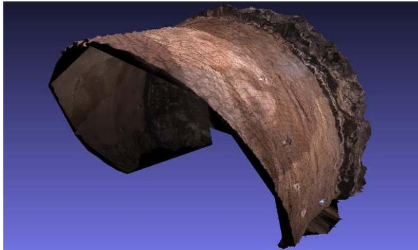
(c) A 3D rendering of the tunnel. The working face is visible in the inside. Immediately before it is the raw tunnel surface as excavated, without shotcrete applied, and therefore has a slightly higher diameter and a rougher surface.
