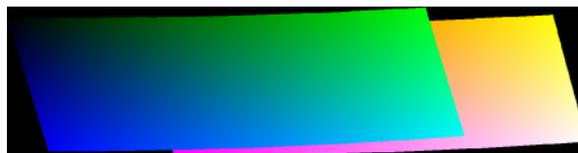
Figure 2.17: Colour coded image mapping for image borders as cut lines. The red channel is the image index, while green and blue encode the location of the pixel in the source image
