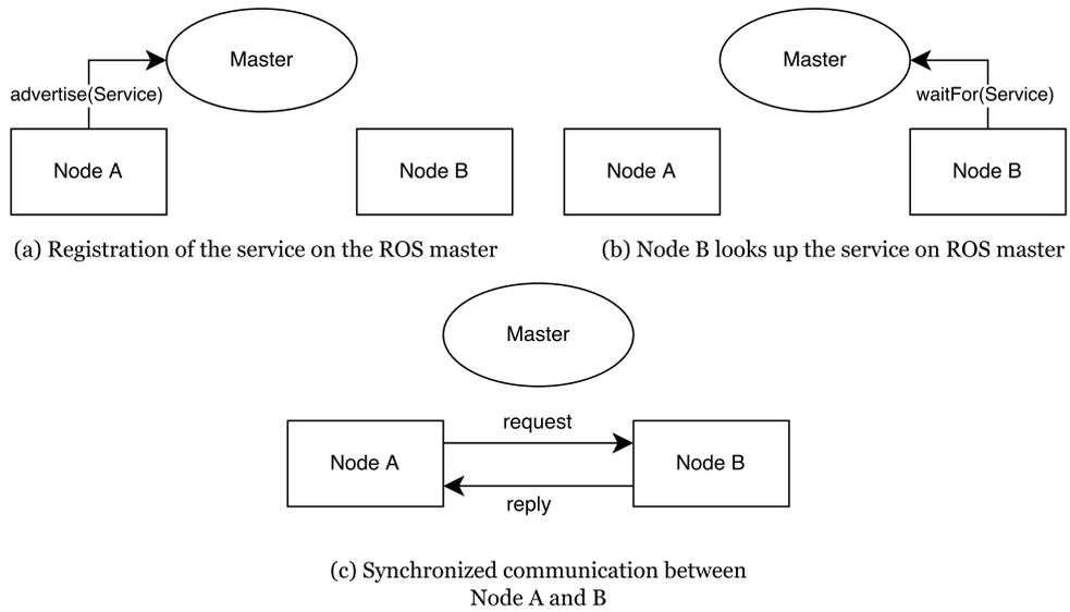
Figure 4.2: Concept of the service model in ROS. Figures adapted from <http://wiki.ros.org/>
