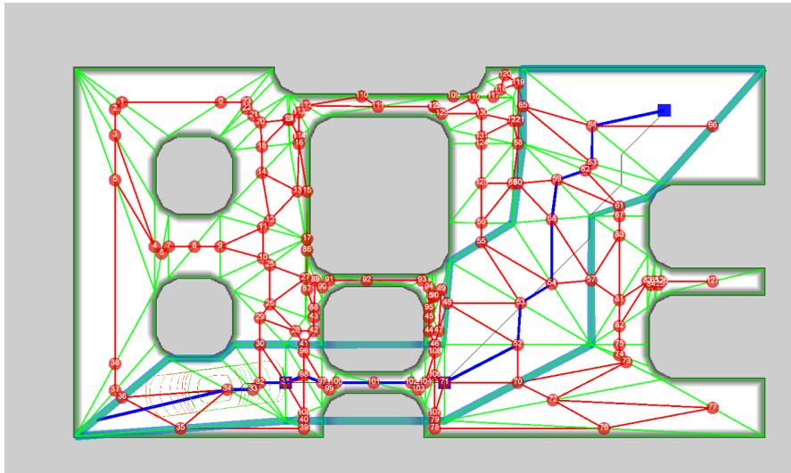
Figure 5.16: Resulting high-level plan for a start goal combination in our running example. (green) visualizes the triangulation and (red) illustrates the road map graph. The high-level plan goes through the empty single robot region: path connecting the waypoints (blue); corresponding planning window (cyan).
