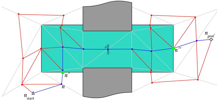
Figure 5.12: The figure presents a small graph through a single robot region. The illustration comprises: a traffic region (cyan); the connectivity graph (red); obstacles (gray); path through the SR region (blue) with entry and exit nodes (green). A\* will eventually choose  $n$  for expansion,  $n$  investigates the node  $n'$ . From the entry node a path is computed through the traffic region until an exit ( $n''$ ) has been determined.
