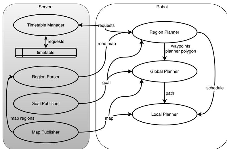
Figure 5.18: Conceptual overview of the navigation system extensions cooperating with the existing navigation stack.
