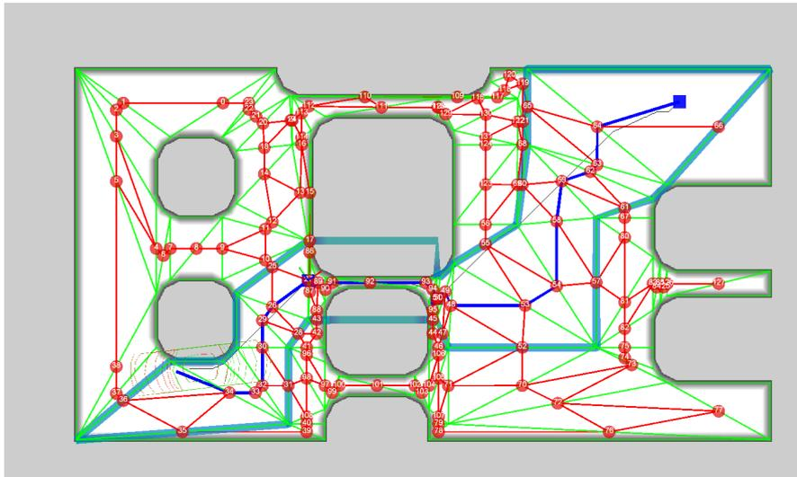
Figure 5.17: Resulting high-level plan for a start goal combination in our running example with a blocked SR region. (green) visualizes the triangulation. (red) illustrates the road map graph. The high-level plan bypasses the blocked single robot region, since waiting in front of the region would take longer than detouring the blocked region: path connecting the waypoints (blue); corresponding planning window (cyan).
