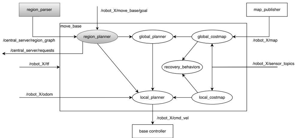
Figure 6.6: Overview of the composition of the extended MoveBase package. (gray) components are novel parts necessary for region planning. Adapted from [http://wiki.ros.org/move\\_base](http://wiki.ros.org/move_base)
