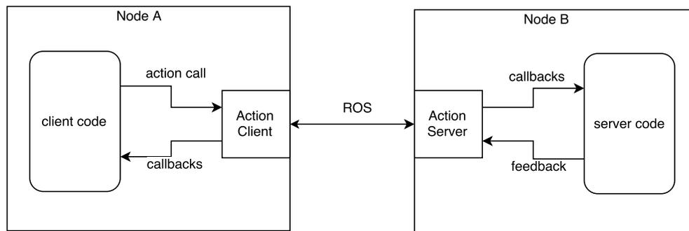
Figure 4.3: Illustration of the action-server and action-client communication. Adapted from <http://wiki.ros.org/>
