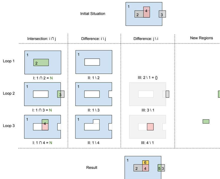
Figure 5.6: Illustration of the Advanced Region Determination Algorithm. This figure shows the sequence of intersection and difference operations to obtain all subregions generated through overlaps. The first rectangle denotes the initial situation. Loop 1-3 shows the effect of the iterations in the inner loop of the algorithm. The first column (I) represents the intersection of the regions. (II) denotes the difference of two regions, while (III) denotes the difference of the exchanged regions.
