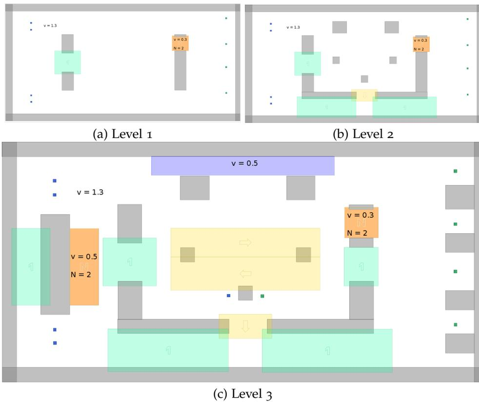
Figure 7.1: Evaluation scenarios with increasing complexity. The variable  $v$  describes the maximal allowed velocity in the corresponding region. The blue and green spots in the free space denotes goal stations. The maps comprises: one ways (yellow); n-robot zone where maximal two robots are allowed (orange); single Robot zone (green); simple traffic areas (blue); forbidden areas (gray)
