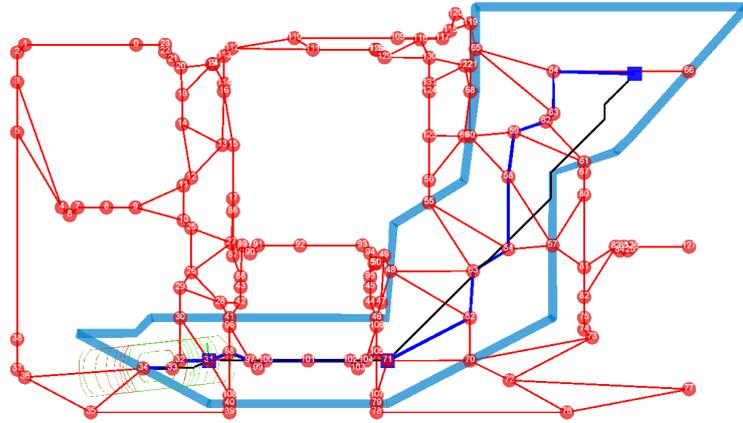
Figure 6.8: Illustration of the region-plan. The region-plan is visualized with the planning window (light-blue) and the path (blue) which connects the waypoints (blue-squares). The *GlobalPlanner* path (black) is respecting the waypoints of the region-plan.
