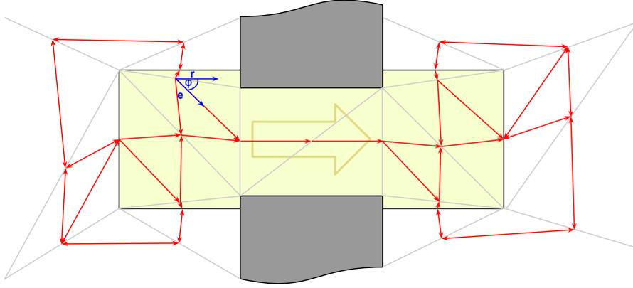
Figure 5.9: Illustration of a resulting graph for an oneway traffic region. The figure denotes the directed edges (red), represents the OW (yellow), indicates a triangulation of the regions (grey) and visualizes the angle test for one specific edge (blue)
