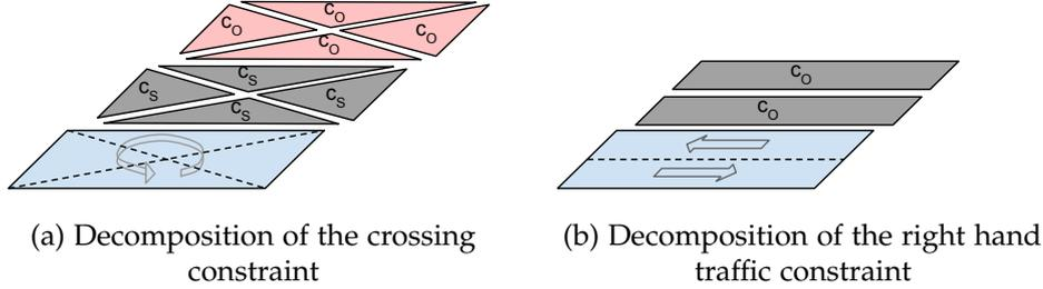
Figure 2.1: Illustration of the constraint decomposition. ( $c_S$ ) denotes the single robot constraints, ( $c_O$ ) shows the one way constraints.
