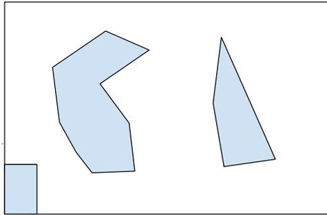
Figure 5.5: Illustration of an exemplary free space polygon (white) with holes, resulting from obstacles (blue) cut-out.
