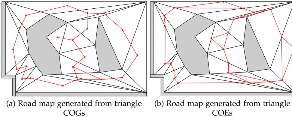
Figure 5.7: Two variants of road map generation with a triangulated polygon. (a) road map generated via connecting neighboring COGs; (b) road map generated via connecting neighboring COEs. Adapted from [22, chap. 6.3.2]
