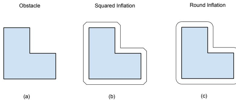
Figure 5.4: Illustration of two obstacle inflation methods. (a) obstacle to be inflated; (b) obstacle inflated with “squared” approximations of all convex edge joins; (c) obstacle inflation with rounded convex edge joins
