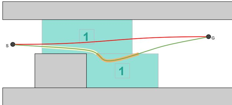
Figure 5.14: Visualization of a scenario with a non optimal plan. The scenario shows two single robot zones (blue) with forbidden areas (gray). The direct path to the goal (red) is shorter but obtains a waiting time due to reservations. The optimal path (green) respects the given reservation scenario and traverses only a part of the upper SRZ.
