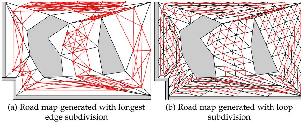
Figure 5.10: Two variants of road map generation (red) with a subdivided triangular-mesh (black triangles). (a) represents the longest edge subdivision. At is clearly visible that graph nodes of large triangles have a very high degree after this subdivision method; (b) dense road map generated via the loop subdivision procedure. This method keeps the low degree of maximal four edges connected to a node.
