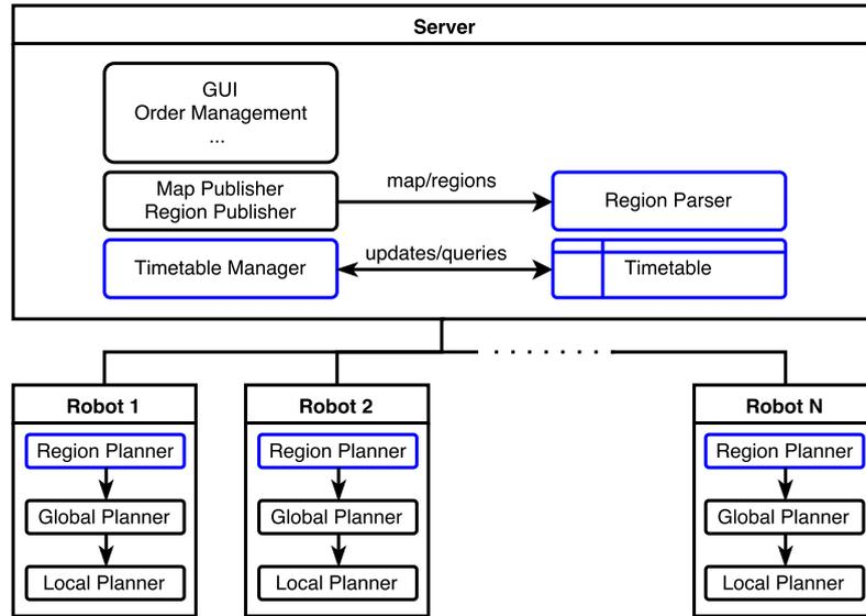
Figure 5.1: Schematic overview of the navigation system. (blue) denotes the novel parts integrated into the existing system (black)
