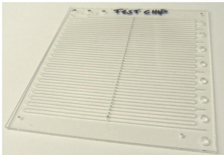
**Figure 5.1:** Polymer microfluidic chip with 40 integrated pH sensor spots of about 350  $\mu\text{m}$  each
