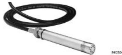
used. The input impedance of Type 2671 is lowered to 1.5 GΩ with the purpose of making a high-pass filter at 20 Hz. This is done in order to compensate for filters which are often missing in the input modules (for example, A-weighting). Type 2671 is also available in a version without the high-pass filter, which has a flat response down to 2 Hz, and in a version with built-in A-weighting, Type 2699.
