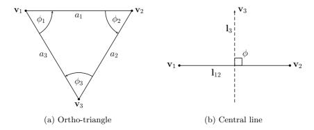
Figure 2.6: Necessary conditions on vanishing points: (a) the ortho-triangle has  $\phi_1 < \frac{\pi}{2}$ ,  $\phi_2 < \frac{\pi}{2}$  and  $\phi_3 < \frac{\pi}{2}$ , (b) square pixel cameras fulfill  $\mathbf{l}_3 \perp \mathbf{l}_{12}$  ( $\phi = \frac{\pi}{2}$ ), whereas  $\mathbf{l}_3$  is the central line with  $\mathbf{l}_3^{\mathsf{T}} \mathbf{v}_3 = 0$  (dotted) and  $\mathbf{l}_{12} = \mathbf{v}_1 \times \mathbf{v}_2$  is a vanishing line.
