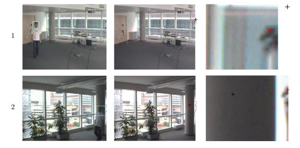
Figure 4.22: Camera localization with Sequence 2 of the Seminar room dataset. Left: Sample face detections that are used. Middle: The estimated epipoles in both cameras. Right: A magnification of the middle images within the red rectangles.
