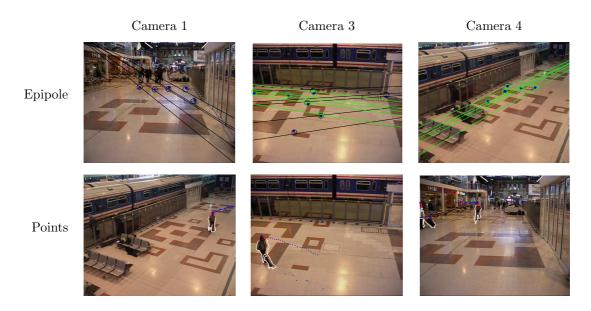
Figure 4.17: (Left column: Results of the camera calibration. The ground truth points are drawn in blue. The circles show the re-projected points. The epipolar lines of the corresponding ground truth points are also drawn. Correspondences between Camera 1 and 3 are shown in black and between Camera 3 and 4 in green. Right column: The output of the head point detector. Blue are the head points. Some outliers can be recognized.
