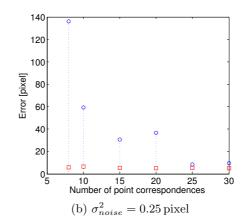
Figure 4.12: Error evaluation with 8, 10, 15, 20, 25 and 30 point correspondences. (a) Zhang's error of our calibration vary around 5.6 pixel (red). The largest error of the 8-point algorithm is 157.04 pixel (blue). (b) The errors of our calibration remain in the same order.
