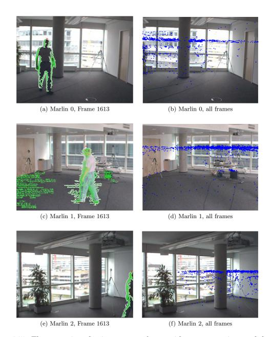
Figure 4.15: The generation of point correspondences with our automatic top of the head detection (red crosses). (a), (c) and (e) show three synchronous images of the three cameras. (b), (d) and (f) show the result as blue points within 2,700 image frames. Notice the outliers and the critical collinearity of the points which has its cause in the room floor restricted motion of people.
