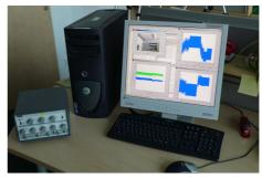
(b) Pulse generator (left) and PC (right)
