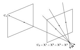
Figure 3.10: Illustration of the configurations that collapse to a meaningless geometry. The reader can see that  $C_2$  and all reconstructed positions of the trajectory are a single point. This is possible, because only one observation of a position in Camera 1 is available.
