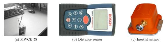
Figure 4.3: Sensors that measure the ground truth. (a) LED light as point light source. The LED MWCE 5571 is extremely bright (460 mcd) and has an angle of reflected beam of 150 deg. (b) A commercial laser sensor from Bosch. The accuracy is  $\pm 0.5$  mm for a distance of 30 m. (c) The inertial sensor. The accuracy in the Euler angles is  $\pm 0.5$  deg.
