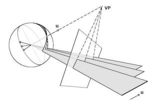
Figure 2.1: The Gaussian sphere [Collins, 1993]. Direction **u** is a point on the sphere which is formed by the great circles of parallel image lines. VP is the vanishing point on the image plane.
