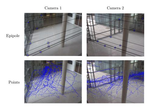
Figure 4.18: The first row shows the correct epipoles and the low error between the manually defined points and their reprojection after triangulation. The worst error was smaller than 3 pixel. The second row shows the point correspondences that are generated by walking people.
