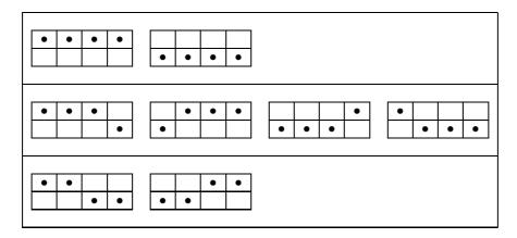
Figure 3.9: Potential minimal configurations. The first row illustrates all observations only in one view which yield no motion parallax. The second row give all combinations of imaged positions where in one view only one observation is available. These configurations all collapse to a meaningless geometry. The third row shows the only remaining configuration which is the correct minimal configuration; two observations in two views.
