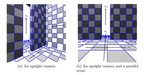
Figure 2.7: Critical cases during camera calibration. The three orthogonal directions are illustrated. (a) vanishing point  $\mathbf{v}_3$  is at infinity in the image plane, (b) vanishing point  $\mathbf{v}_2$  and  $\mathbf{v}_3$  are at infinity in the image plane.
