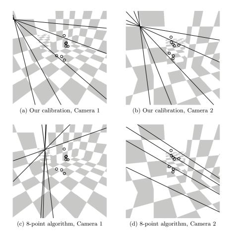
Figure 4.11: An experiment with eight particular point correspondences shown as black circles. (a) and (b) show the black epipolar lines of our calibration. (c) and (d) show the wrong result of the 8-point algorithm. The eight points in each image are neither collinear nor coplanar.
