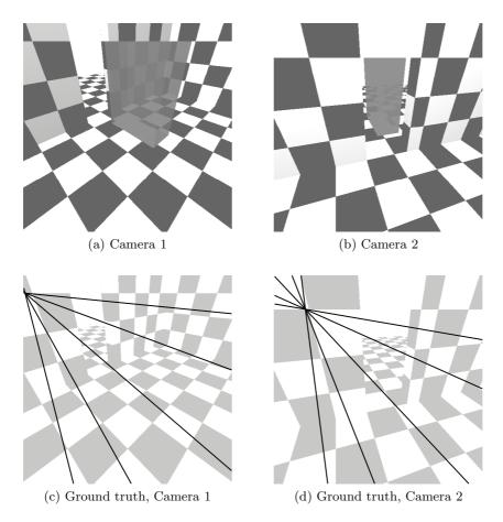
Figure 4.10: Synthetic images of two virtual cameras with small visible overlapping views designed with PovRay which is a raytracing software and is freely available under http://www.povray.org. The highlighted volumes in (a) and (b) are the space where point correspondences are generated. (c) and (d) show the black ground truth's epipolar lines.
