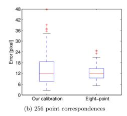
Figure 4.13: Error evaluation with a  $\sigma_{noise}^2 = 1$  pixel. Notched box plots are shown. (a) shows a large error for the 8-point algorithm while in (b) this error reduces drastically but despite is larger than the error of our calibration which was not much affected by the number of point correspondences.
