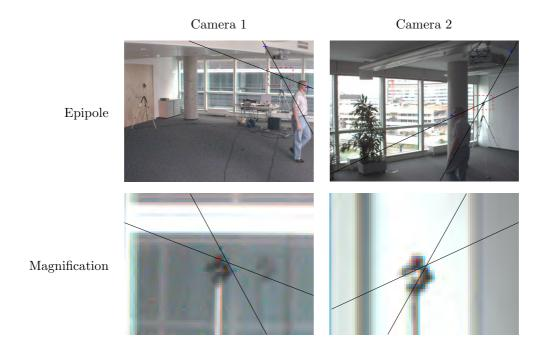
Figure 4.16: The epipoles in Sequence 1 of the Seminar room dataset. The error in the image between the ground truth and the estimates were 3.54 pixel for Camera 1 and 2.96 pixel for Camera 2. The largest error between the manually defined points in the background and their corresponding epipolar lines is 6.27 pixel (the nose in Camera 2). The smallest error was 0.95 pixel (point on ceiling in Camera 1).
