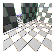
Figure 2.5: The intersection points of three (M=3) concurrent line segments (black, brown, green) are identified. The remaining outlier line segments are drawn in blue.  $\sigma$  was set to 1 pixel. Obviously t is too large, because some line segments belong to the wrong concurrent lines or are spuriously identified as noise.
