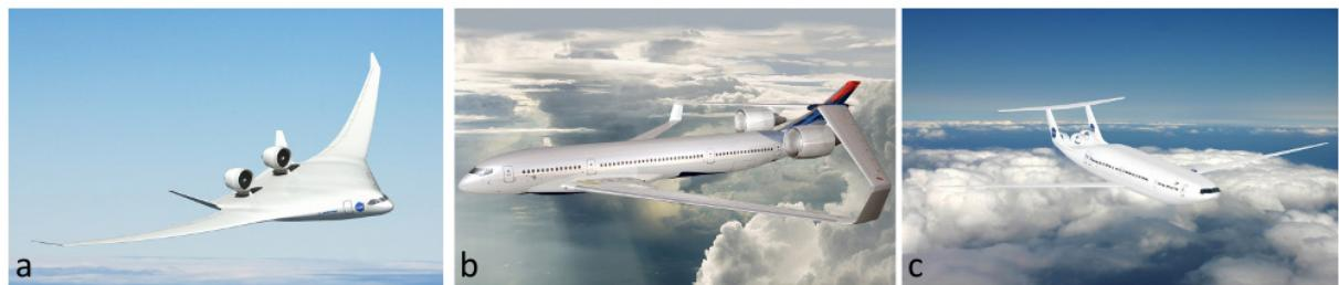
*Figure 1.1: Future aircraft concepts: (a) blended wing body (Boeing), (b) box wing (Lockheed) and (c) "double bubble" design (MIT<sup>1</sup>); [3]*
