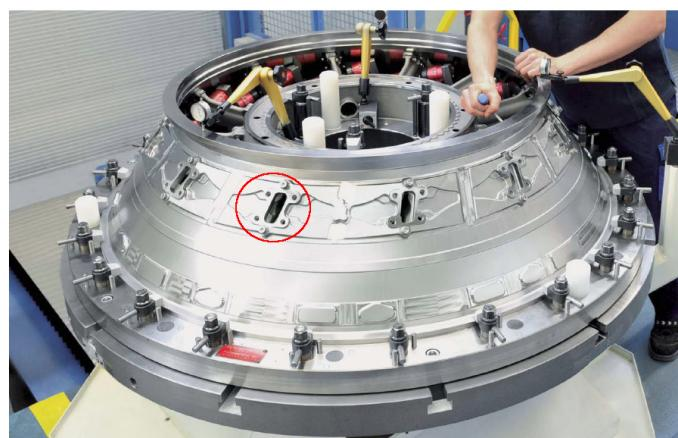
Figure 1.7: Mid turbine frame of the GEnx jet engine (General Electric); [9]
