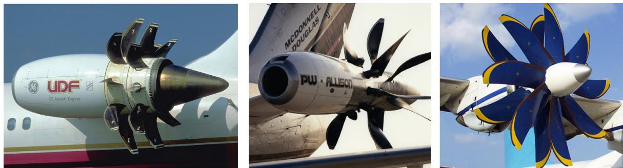
Figure 1.4: Open rotor concepts in the 1980's from General Electric (GE-36), Pratt and Whitney (578-DX) and Iwtschenko Progress (Progress-D27)
