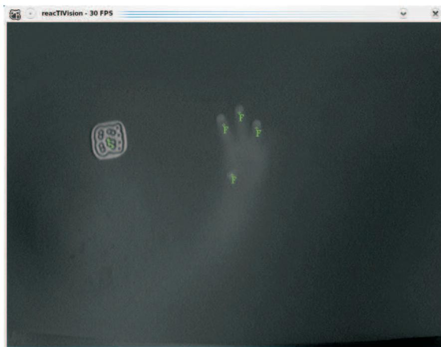
Figure 14: Recognition of fiducial symbol and finger events
