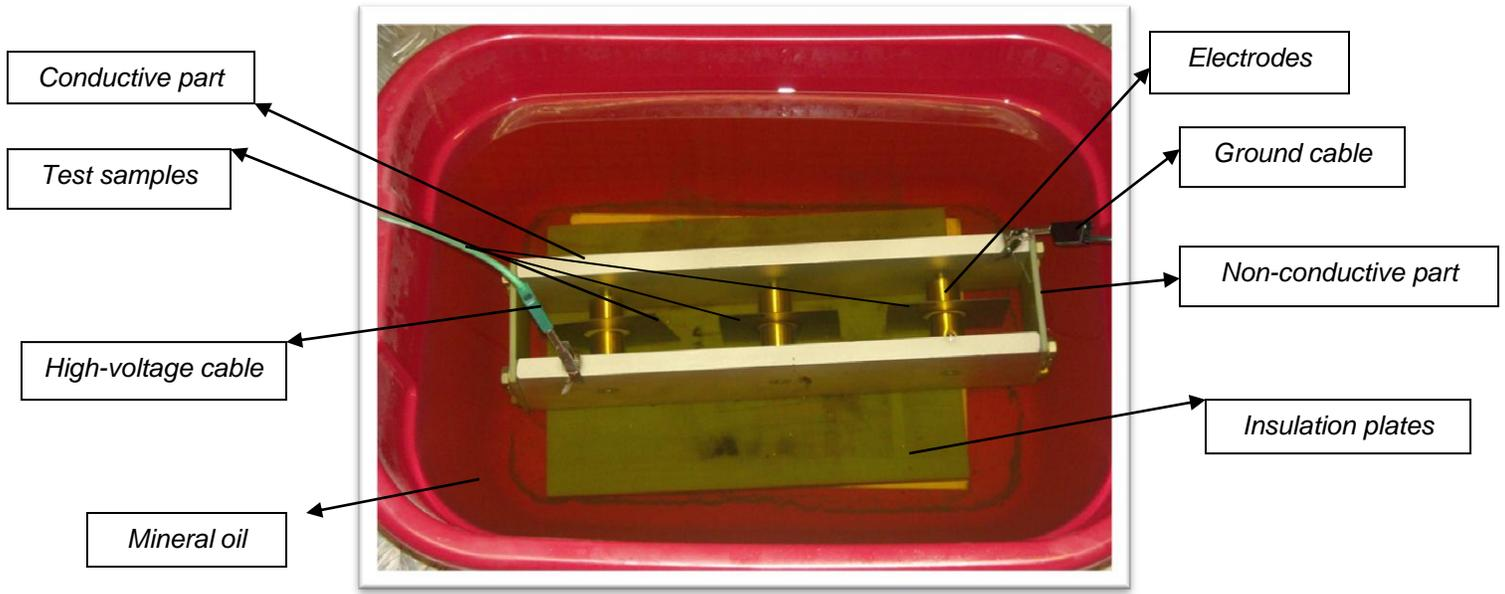
Picture 16: Van with mineral oil and test samples between electrodes
