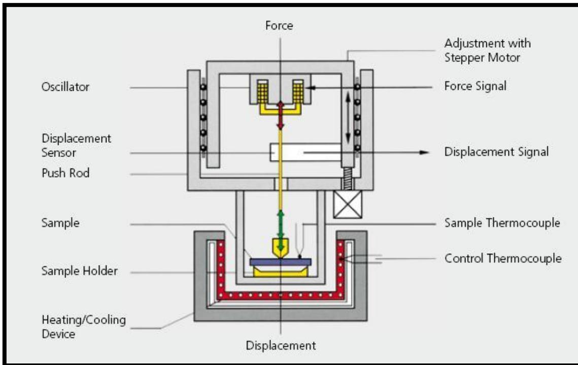
Figure 18: DMA device – construction (15)
