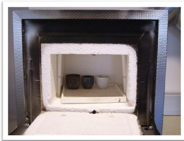
Picture 17: Oven for burning out the organic parts
