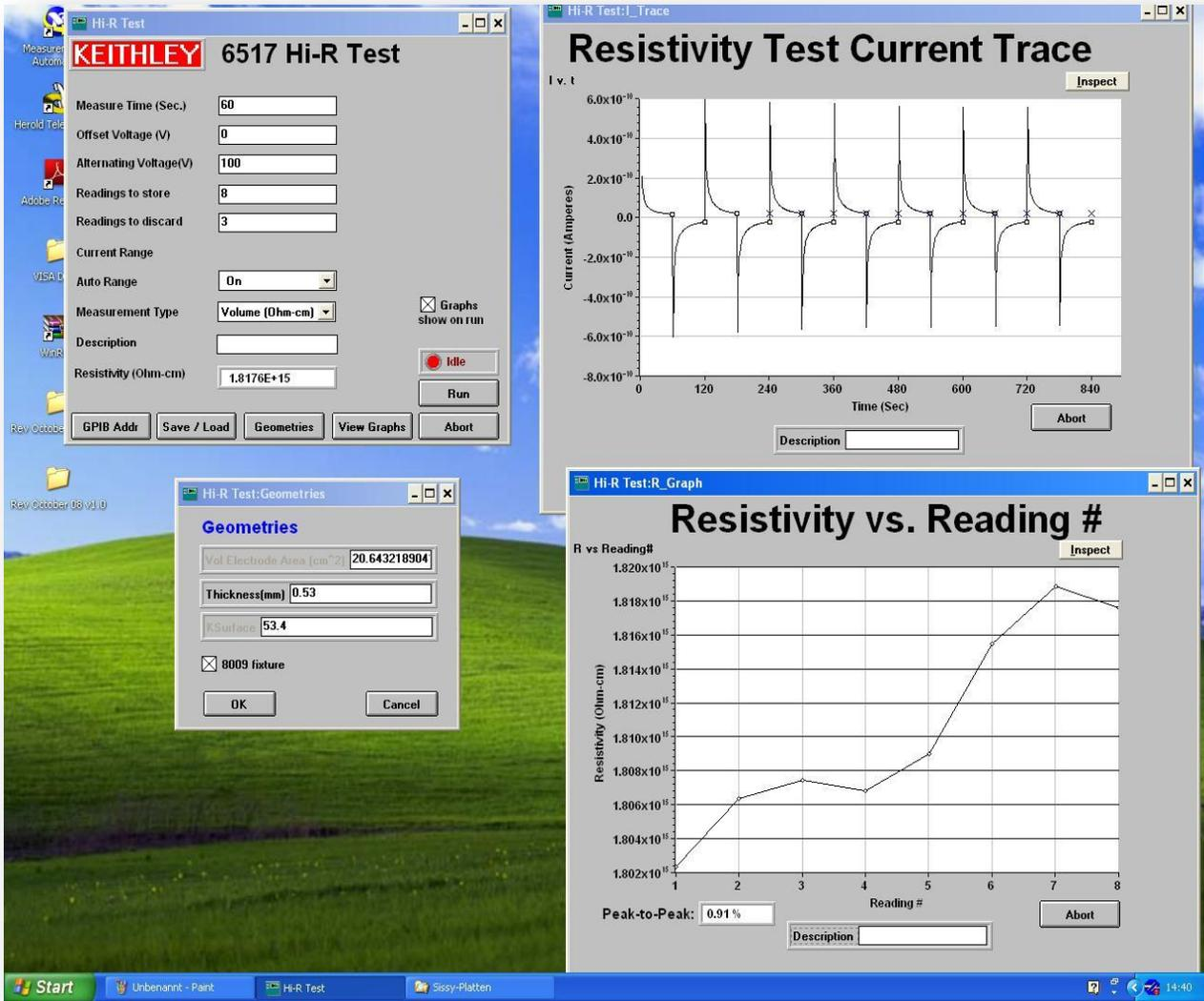
Picture 19: Measurement of a Volume resistivity
