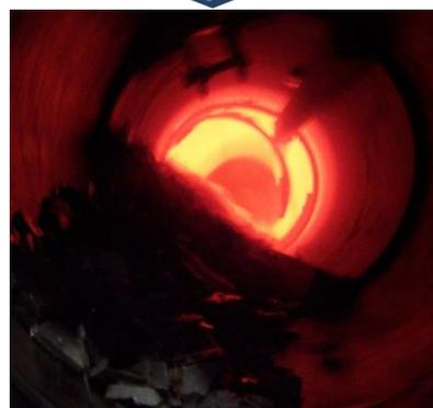
*Mica is heated at 550°C -650°C into a kiln*
