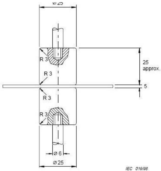
Figure 1b – Equal diameter electrodes
