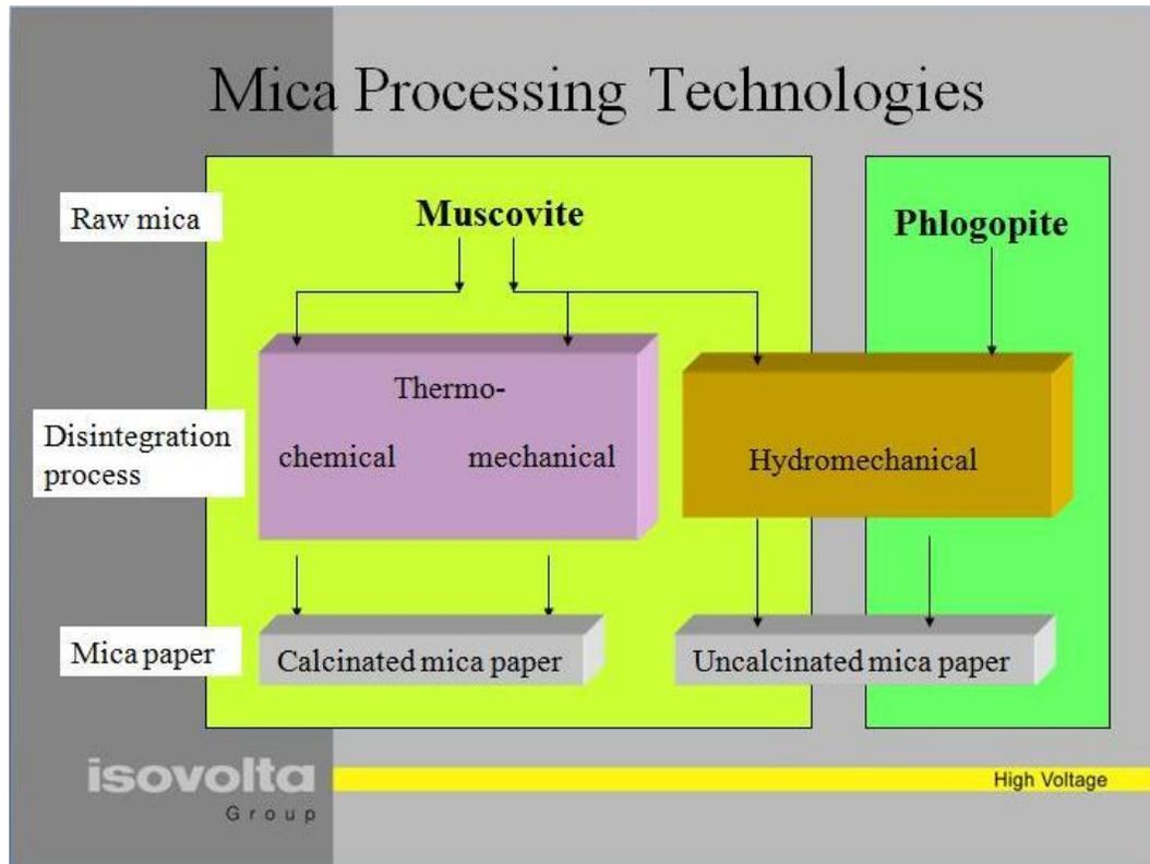
Figure 1: Mica process technology (6)
