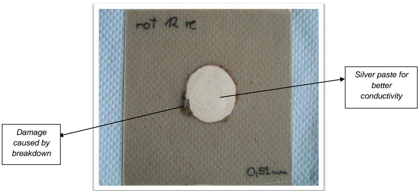
Picture 14: Calmicaglass®0409 after breakdown and a couple of hours under 45kV.
