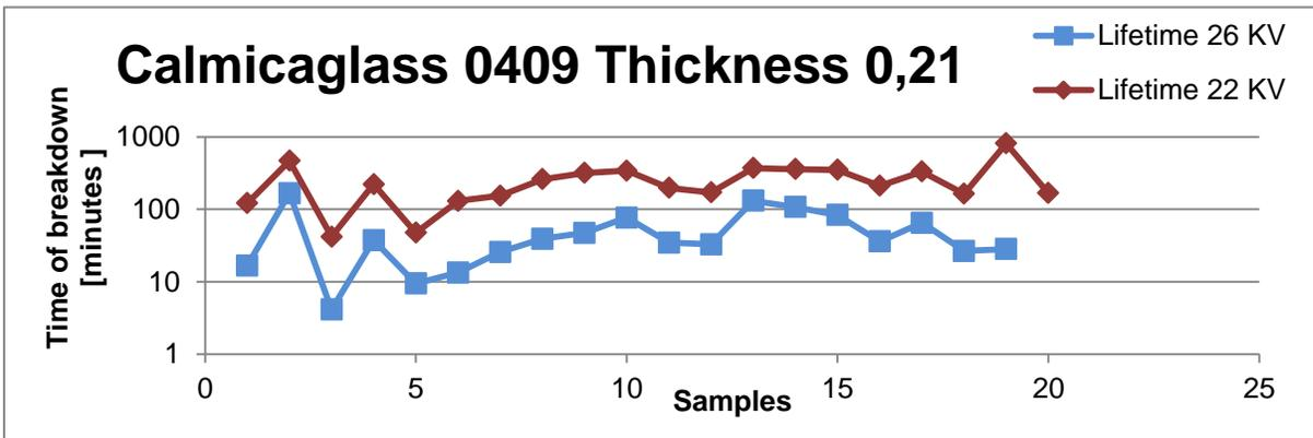
Figure 9: Calmicaglass®0409 thickness 0,21mm
