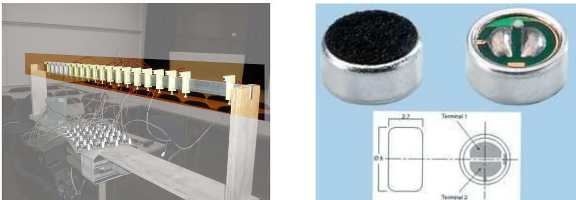
Figure 5.2: microphone array consisting of 20 sub-miniature electret microphone cartridges
