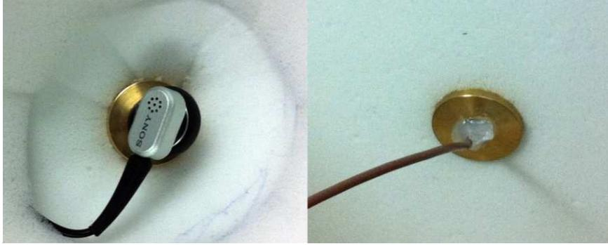
Fig. 3.37 Acoustic Coupler front and back view with IEM
