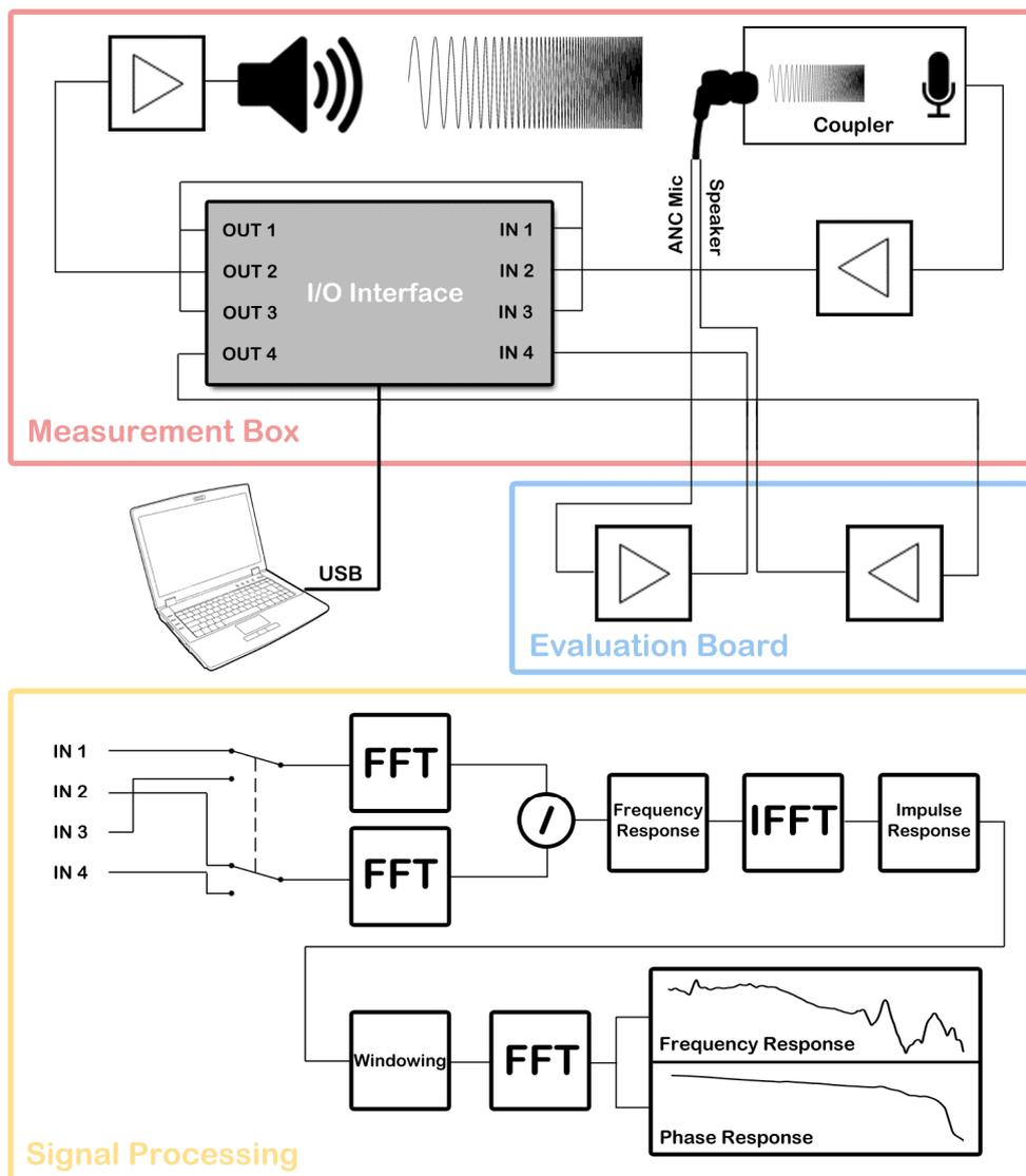
Fig. 5.1 Flowchart, complete measurement system in use with FCT.exe
