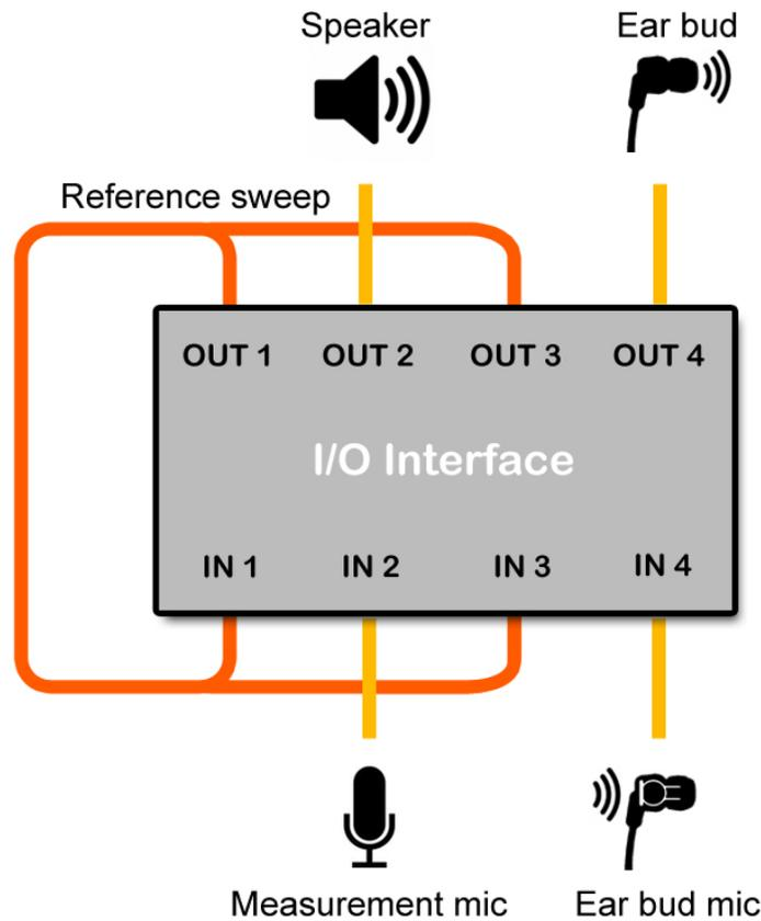
Fig. 4.4 I/O soundcard routing
