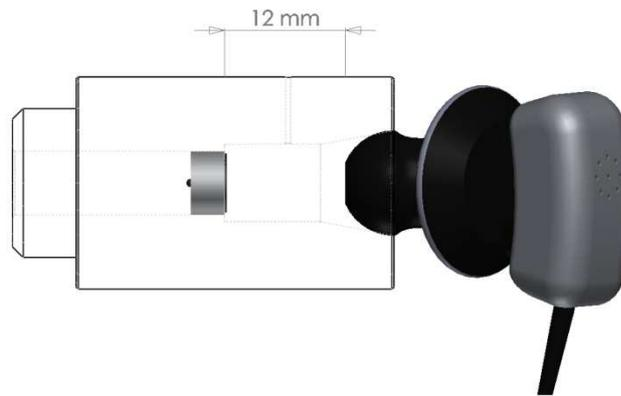
Fig. 3.16 Design drawing, acoustic coupler prototype 2
