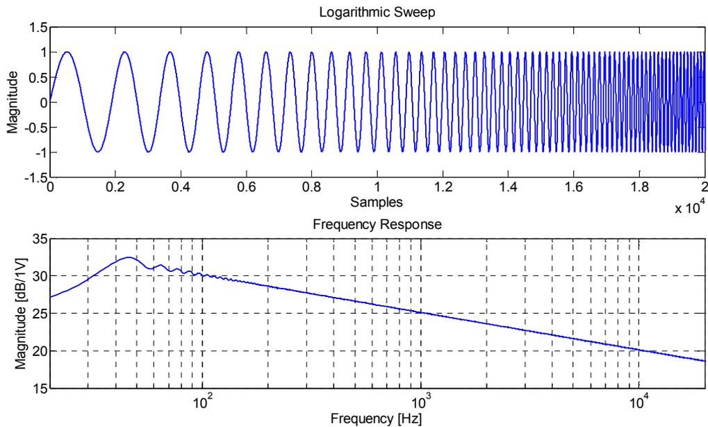
Fig. 2.17 Exponential sweep - Time domain (top), Magnitude spectrum (bottom)
