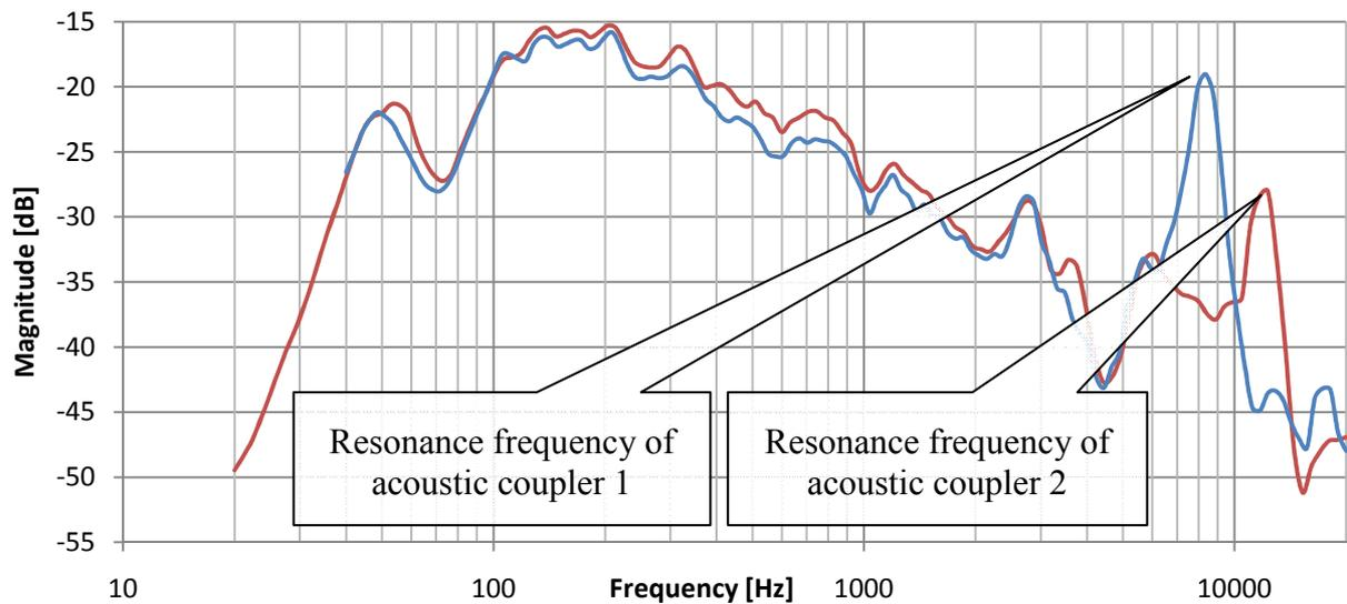
Fig. 3.18 Passive attenuation comparison prototype 1 and 2
