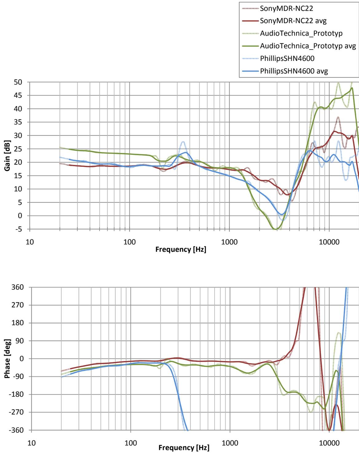
Fig. 3.49 Filter Gain and Phase of 3 different IEM's
