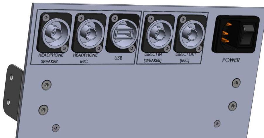
Fig. 5.8 Connector panel
