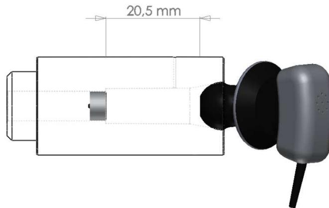
Fig. 3.10 Design drawing, acoustic coupler prototype 1
