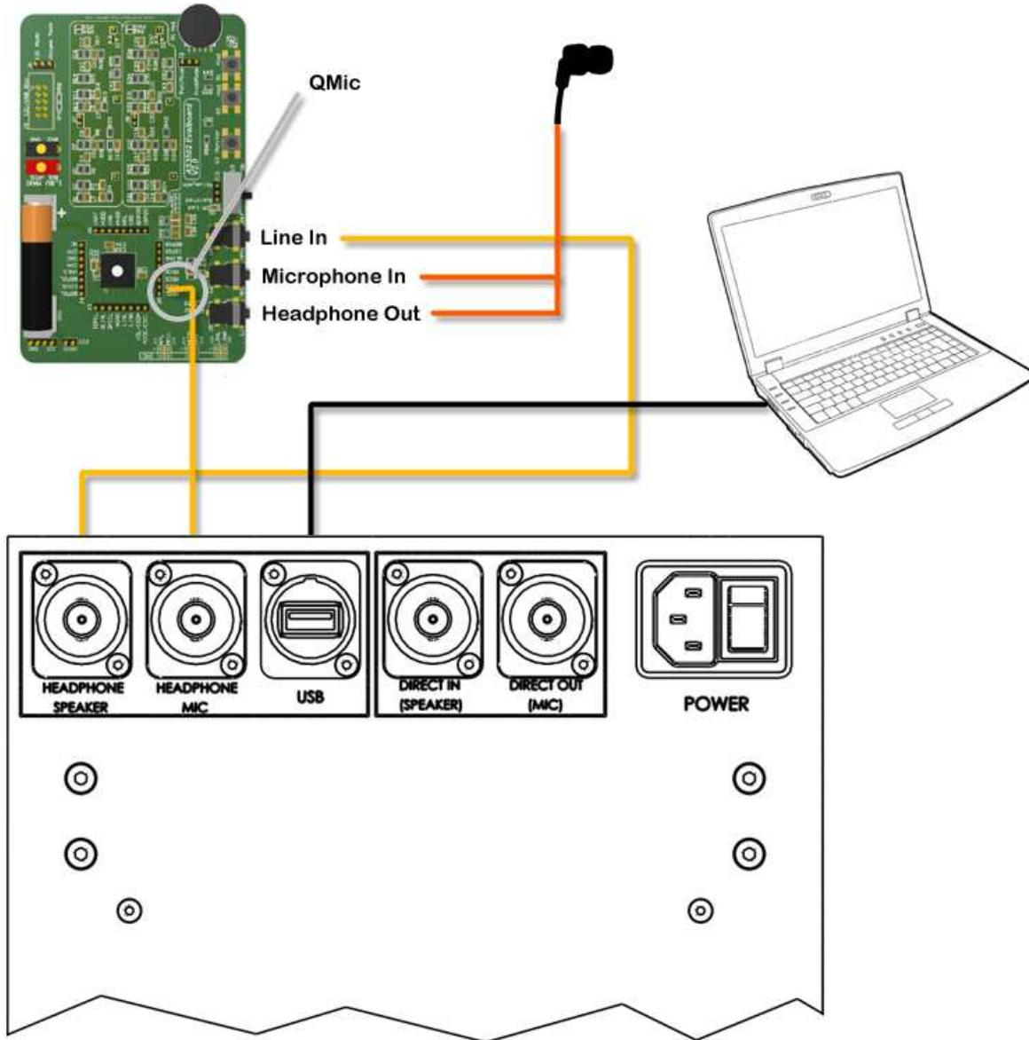
The jacks **Direct In (Speaker)** and **Direct Out (Mic)** provide direct access to the built-in speaker and the measurement microphone. The speaker signal has to be a line signal because the speaker input points at the amplifier. The microphone output provides a pre-amplified signal, too.
