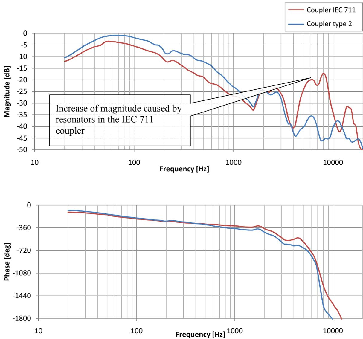
Fig. 3.20 Passive attenuation measurement
