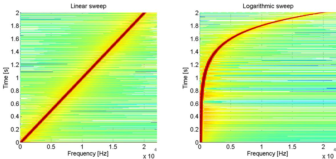
Fig. 2.18 Frequency response over time, linear and exponential sweep
