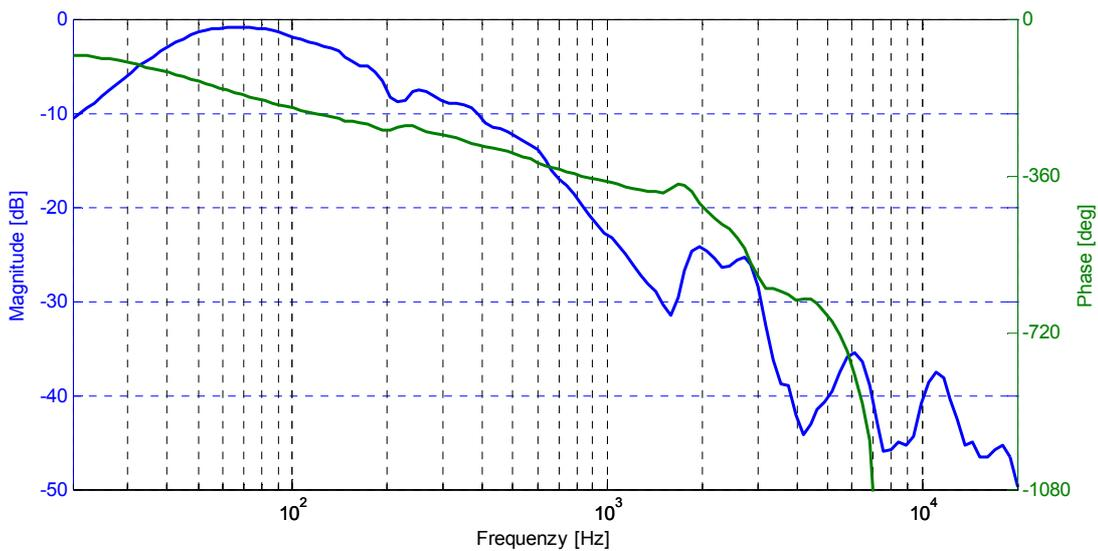
Fig. 2.9 Typical filter gain and phase response, passive attenuation
