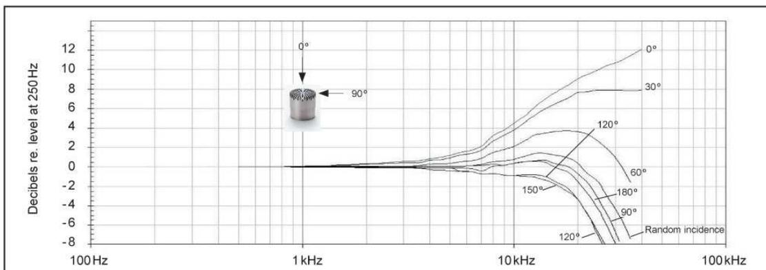
Fig. 3 Free-field corrections for various angles of incidence
