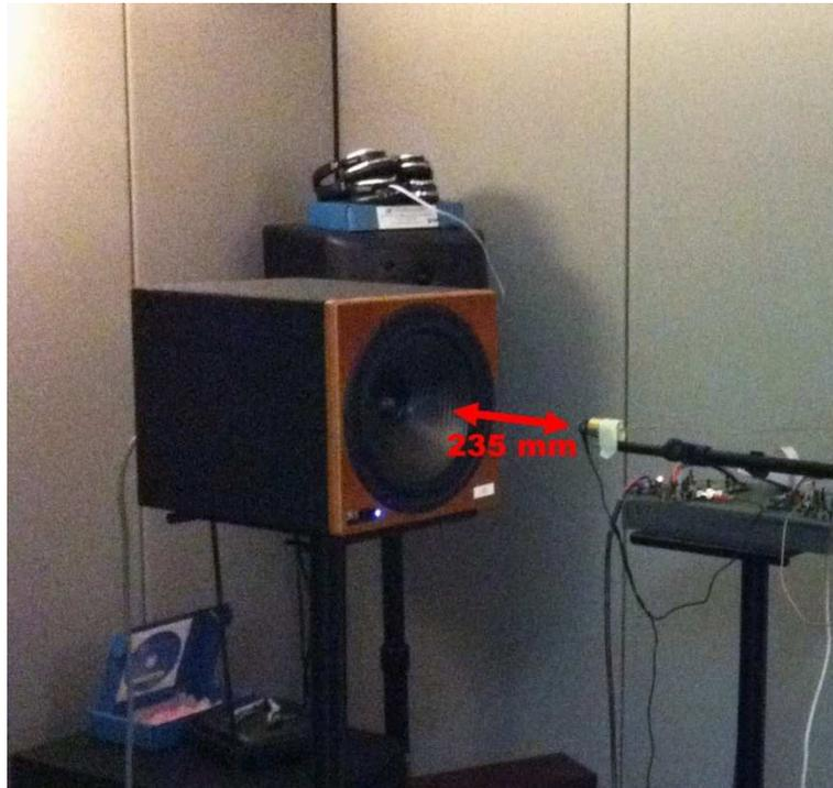
Fig. 3.6 Measurement setup
