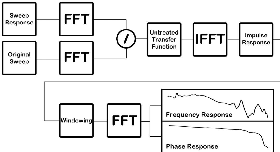
Fig. 2.19 Signal processing flowchart for fft based sweep measurements
