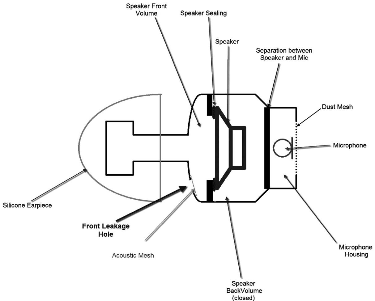
Fig. 2.3 Reference design of an ANC – IEM
