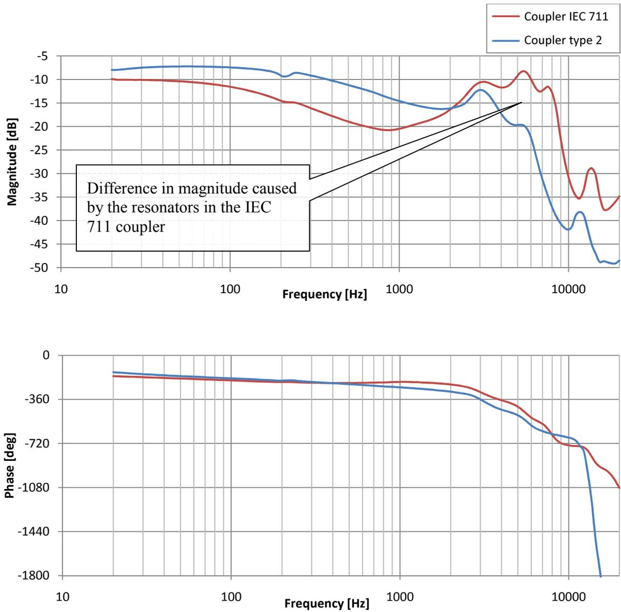
Fig. 3.22 IEM to measurement microphone
