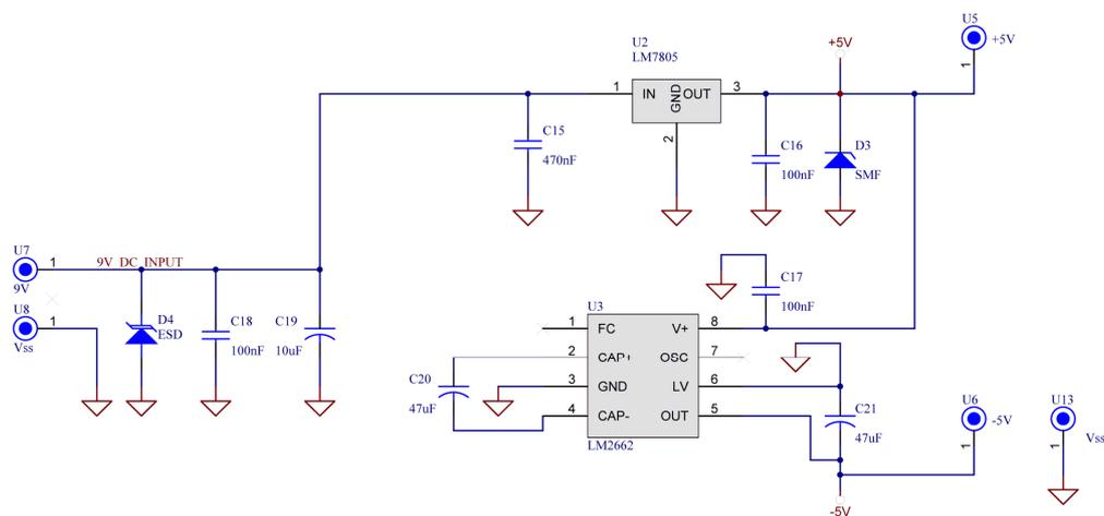
Fig. 3.4 Schematic power supply microphone pre - amplifier
