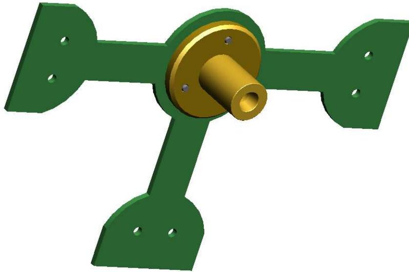
Fig. 5.7 PCB with mounted acoustic coupler
