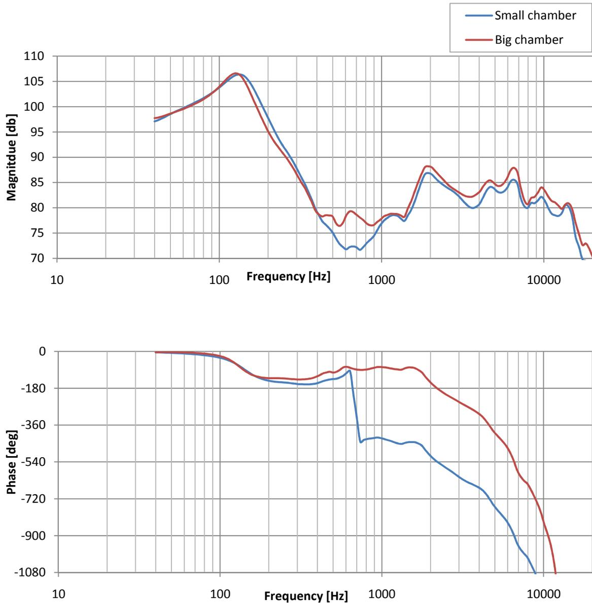
Fig. 3.30 Comparison of small and big chamber
