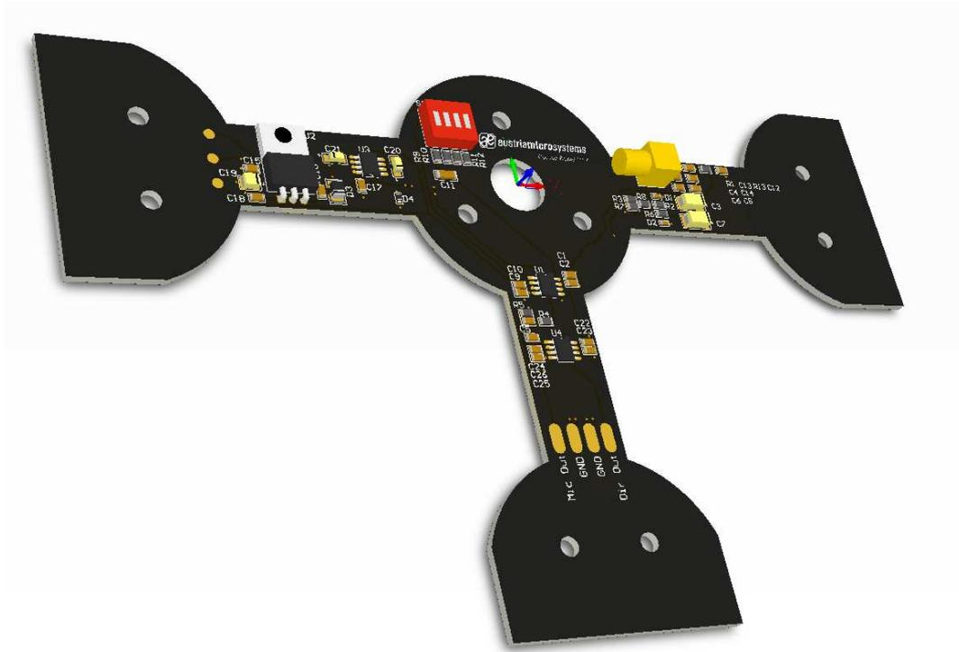
Fig. 3.3 3D model – PCB backside with pre-amplifier circuit
