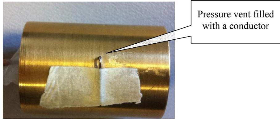
Fig. 3.8 Acoustic coupler with pressure vent
