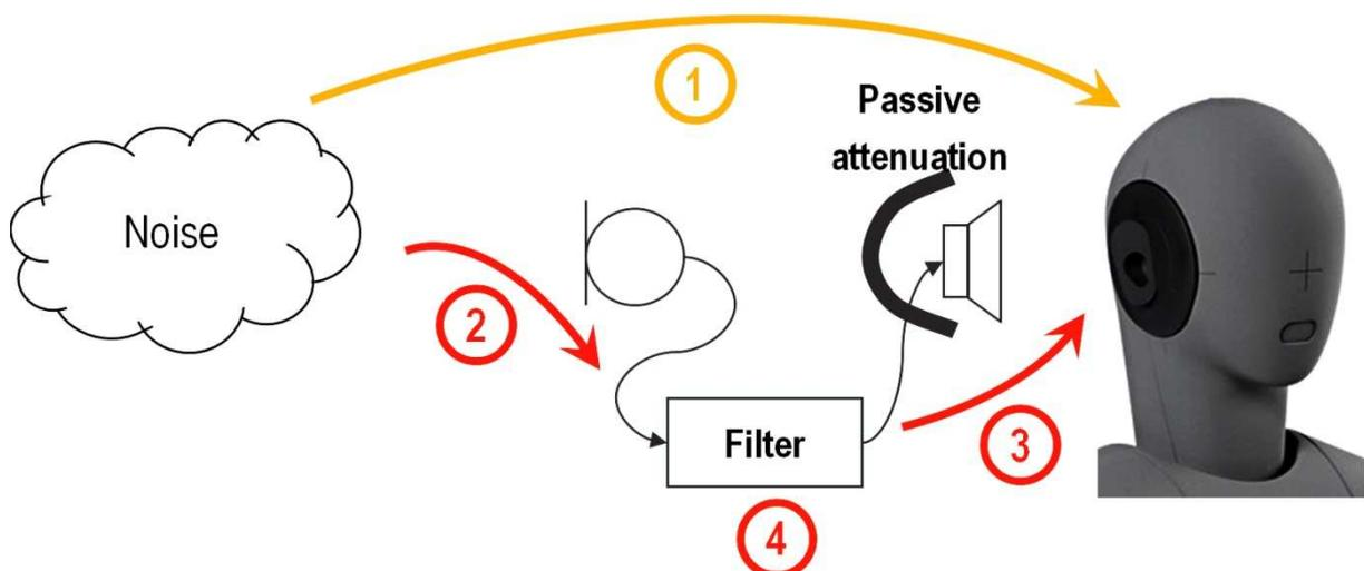
Fig. 2.8 Active and passive noise path
