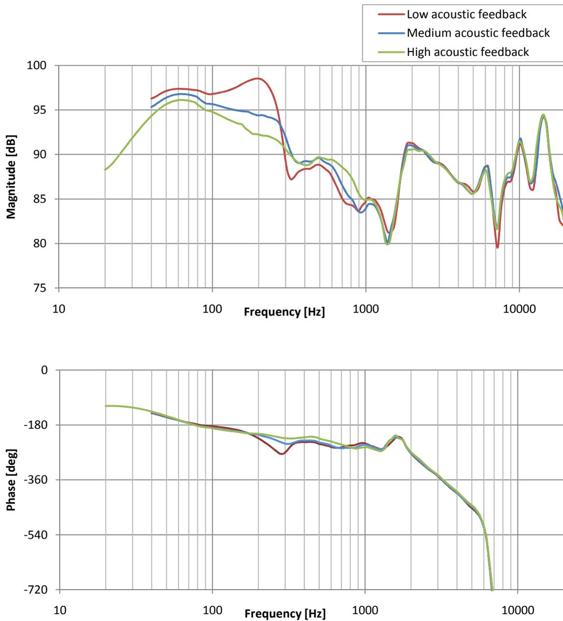
Fig. 3.32 Frequency and phase response of different acoustic feedback plates
