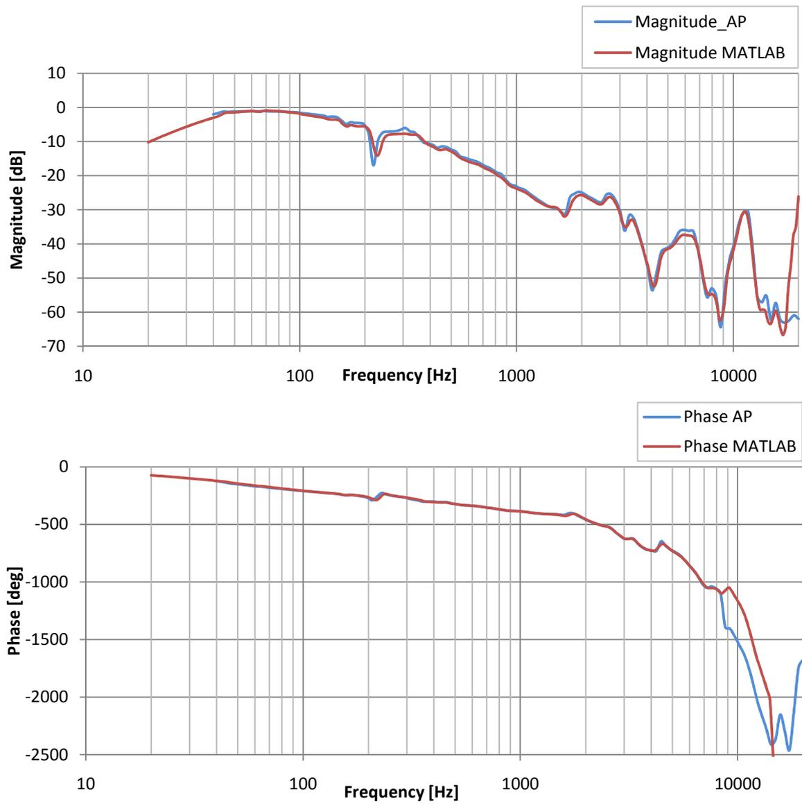
Fig. 4.6 Frequency and phase response, passive attenuation
