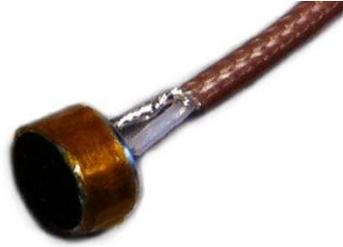
Fig. 3.2 Adapted measurement microphone Panasonic WM-61A
