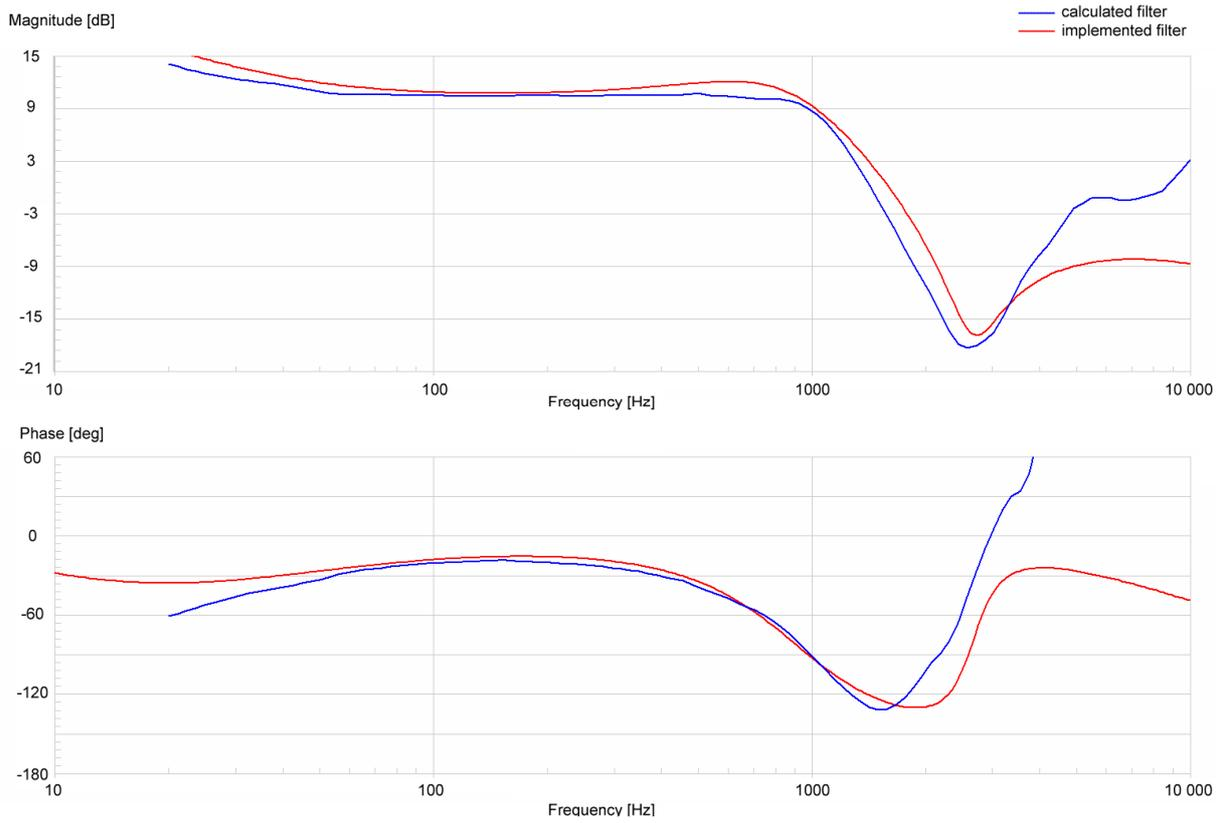
Fig. 2.13 Calculated filter vs. implemented filter
