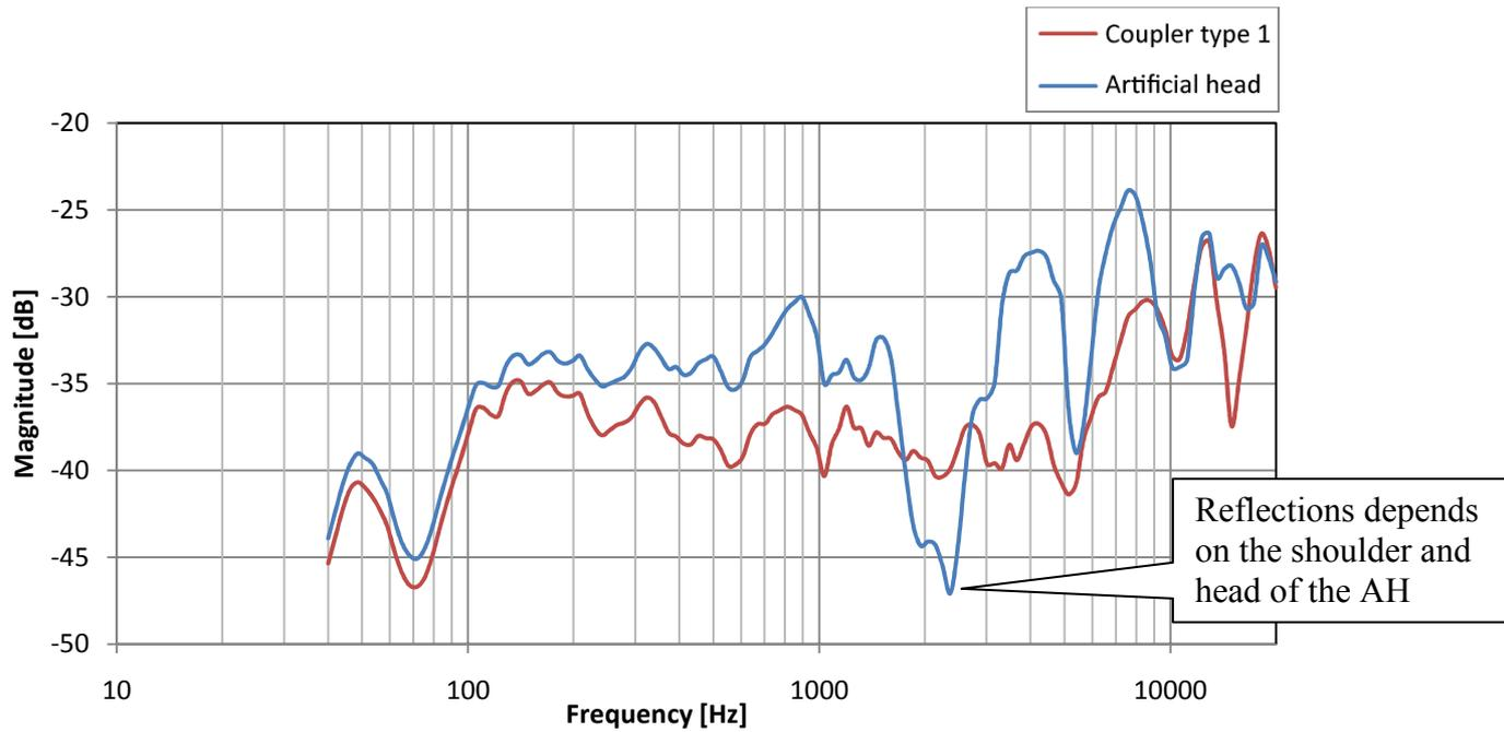
Fig. 3.13 Noise to ANC microphone measurement
