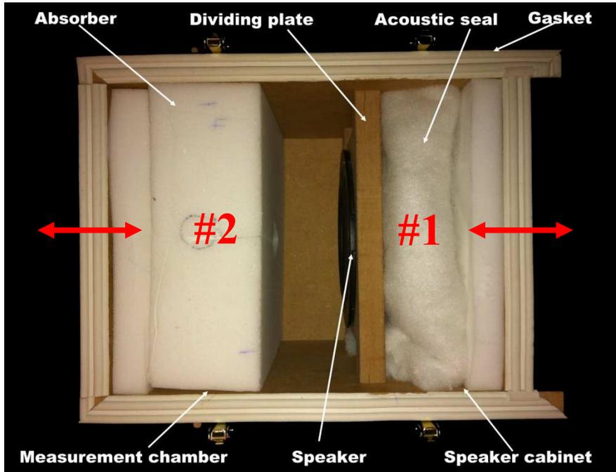
Fig. 3.25 Measurement box inside
