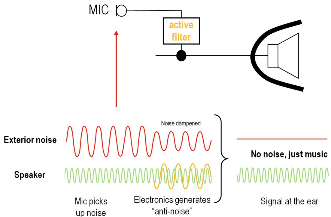
Fig. 2.7 Principles of feed-forward ANC
