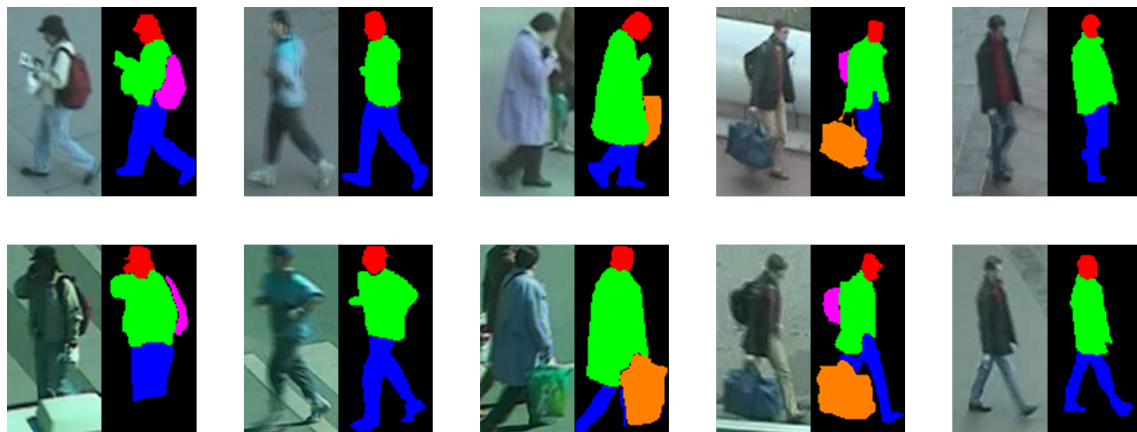
Figure 5.4: Examples from the PRID 450S dataset: Person images and part-level segmentations are shown next to each other. Upper and lower row correspond to appearances of the same person in different camera views.
