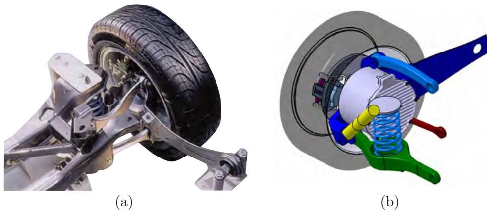
Figure 6.8.: Original control blade suspension system for the rear axle of the Ford Focus from 1999 [HEG11] (a). CAD-model of the control blade suspension system for the rear axle of passenger vehicles with in-wheel motors obtained with the approach presented in this work (b). A 16" rim is used.
