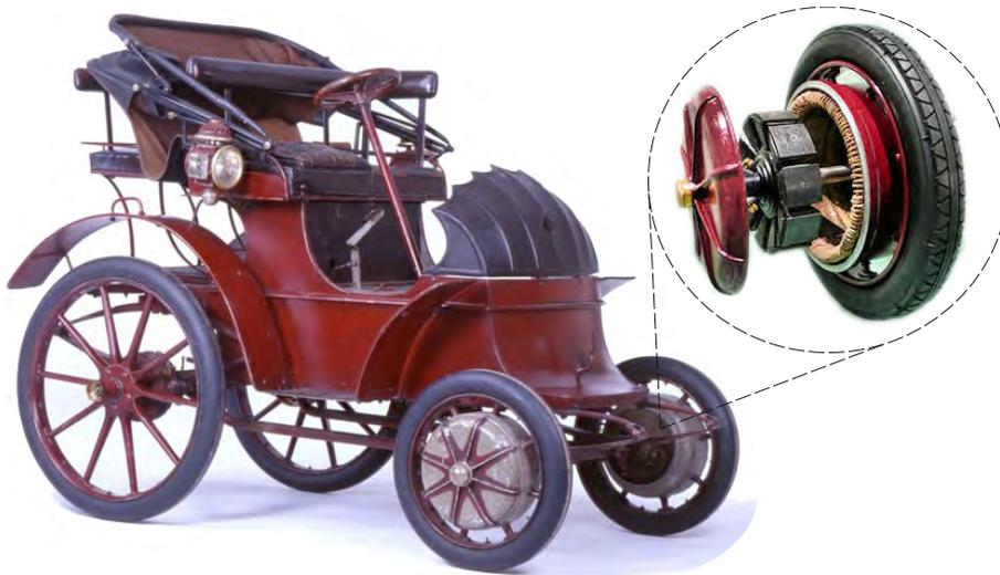
Figure 1.6.: Lohner-Porsche "Semper Vivus": Pure electric vehicle with two DC-in-wheel motors mounted on the front wheels.
