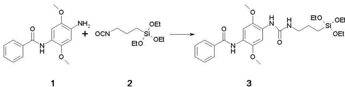
**Figure 18: Fast Blue RR (1) coupled to 3-(triethoxysilyl)propyl isocyanate (2) resulting in the stable urea product (3).**
