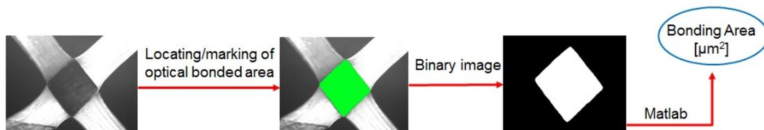
**Figure 3.16:** Determination of the optical bonded area.
