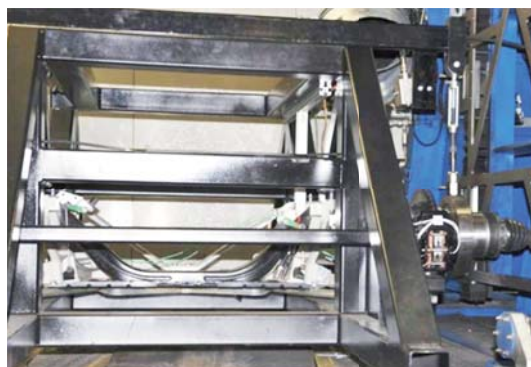
Figure 4.14.: Test set-up showing the test rack at the test bench for NVH investigations.
