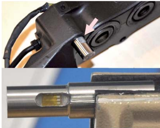
Figure 4.4.: Modified guide pin for friction force measurement.
