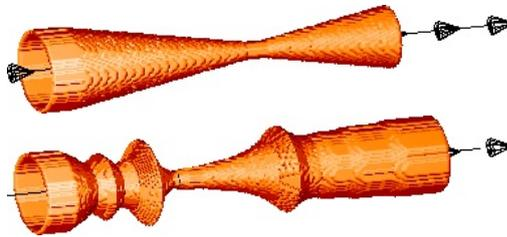
Figure 1.4: Starting solution and final nozzle shape optimized by evolutionary strategies<sup>3</sup>
