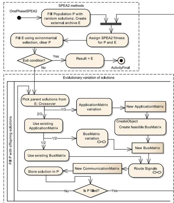
Figure 3.11: Flow diagram of the OnePhaseSPEA2 heuristic
