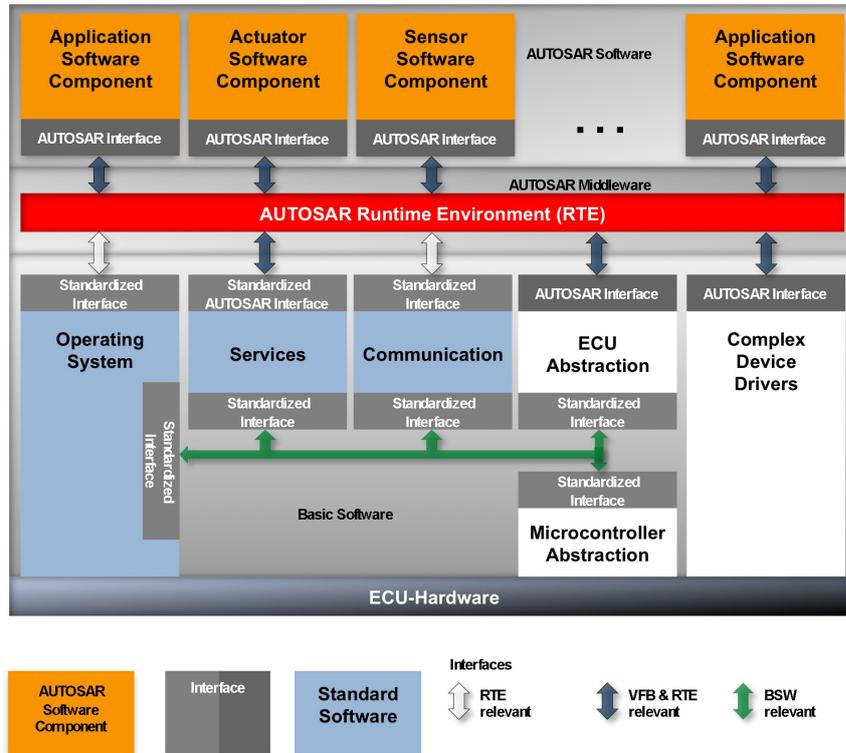
Figure 1.2: AUTOSAR ECU software architecture [23]
