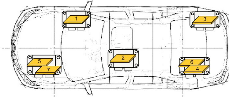
Figure 3.6: An example of mapping of software components onto ECUs
