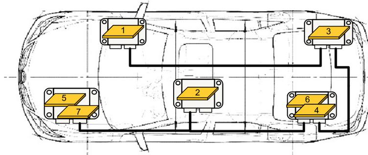
Figure 3.7: An example of connections of ECUs and bus networks
