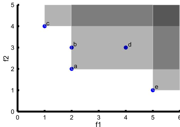
Figure 1.6: Plot of Pareto optimal solutions and dominated objective space
