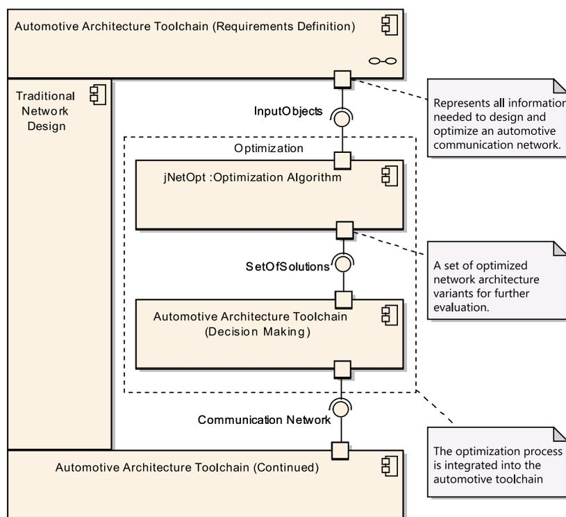
Figure 2.1: Integration of network optimization in E/E architecture development process
