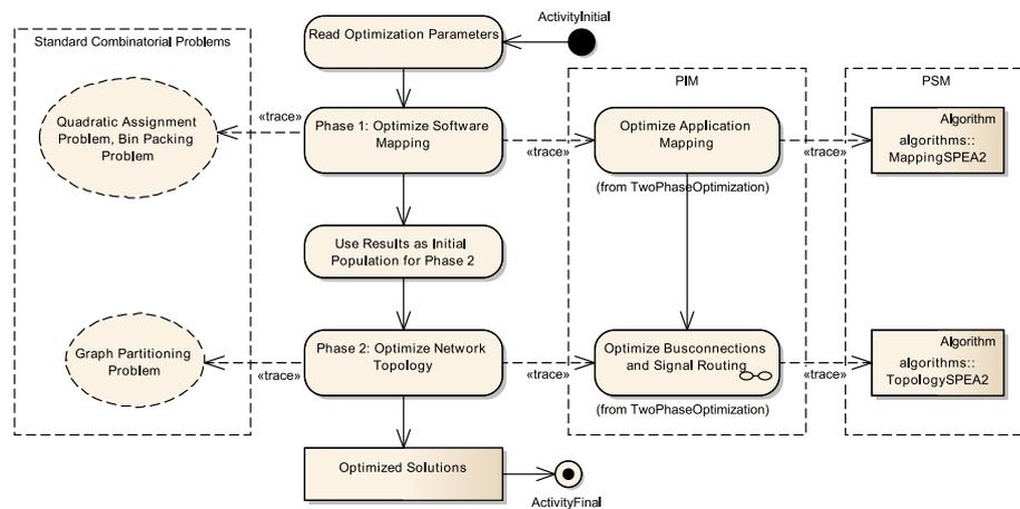
Figure 3.4: Overview of the two-phase optimization approach
