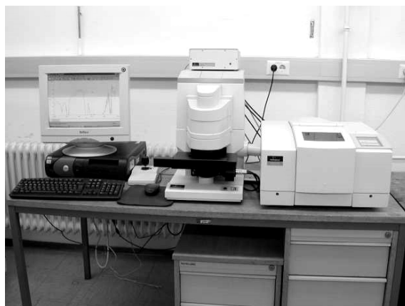
Figure 68: Perkin Elmer 'Spectrum One' FTIR microscope at the Institute of Polymeric Materials, University Leoben, Austria. (Image from http://ssfp.unileoben.ac.at/FTIR.htm )
