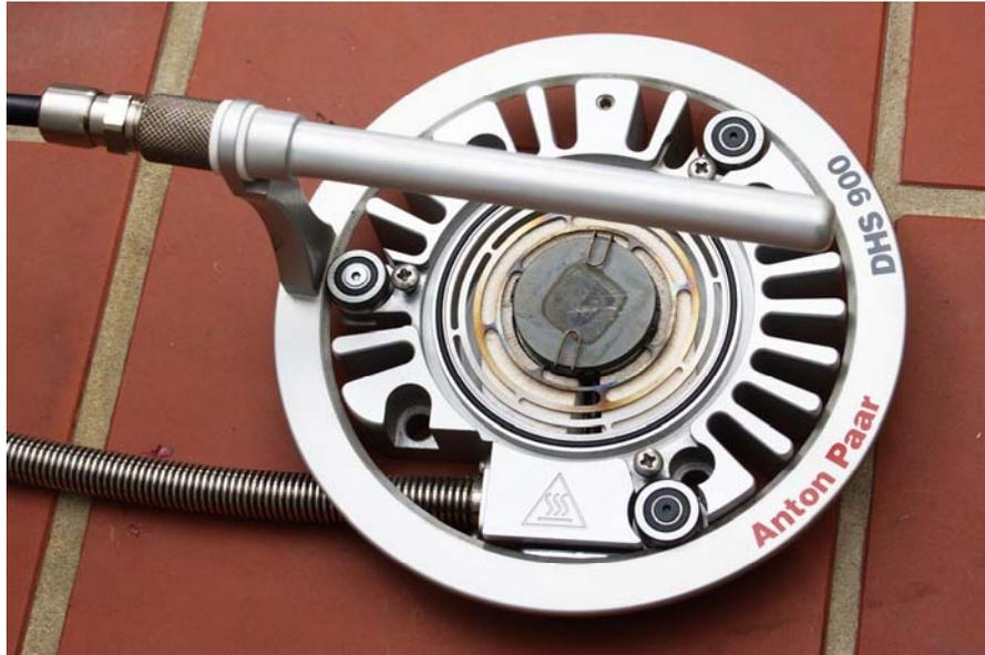
**Figure 3.9) The DHS 900 heating stage. The wafer is placed onto the middle of the stage and can be fixed with the clamps.**
