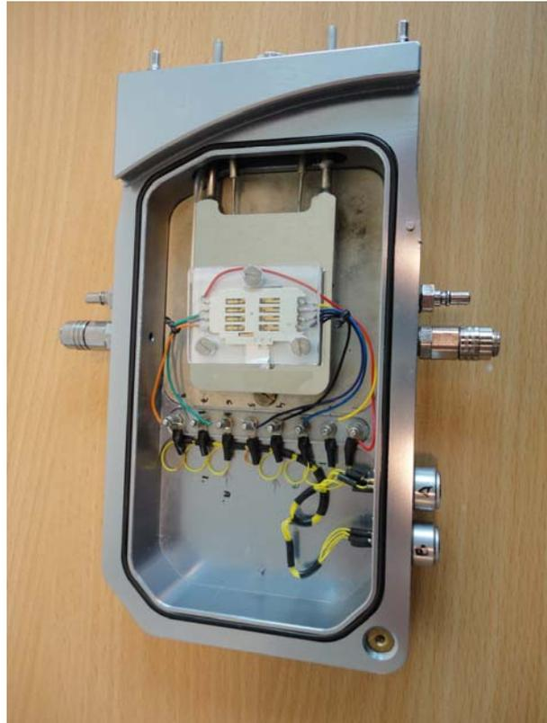
**Figure 3.11) Closer look into the inside of the cooling/heating stage. In the middle the Simcard holder can be seen.**
