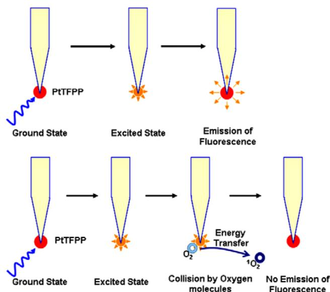
**Fig. 31.** Principle of fluorescence quenching (fluorescent die by oxygen) ([Yinglang et. al., 2011](#))
