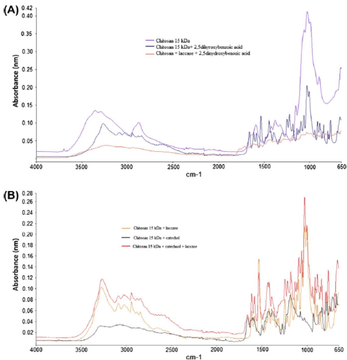
*Fig. 27. FTIR spectra of 2,5-dihydroxybenzoic acid and catechol functionalized chitosan*
