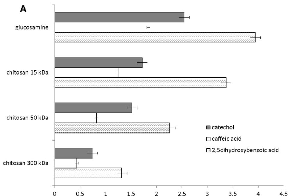
**Fig. 26A.** Consumption of  $-\text{NH}_2$  groups during enzymatic coupling of phenolic molecules to glucosamine and chitosan with different molecular weights
