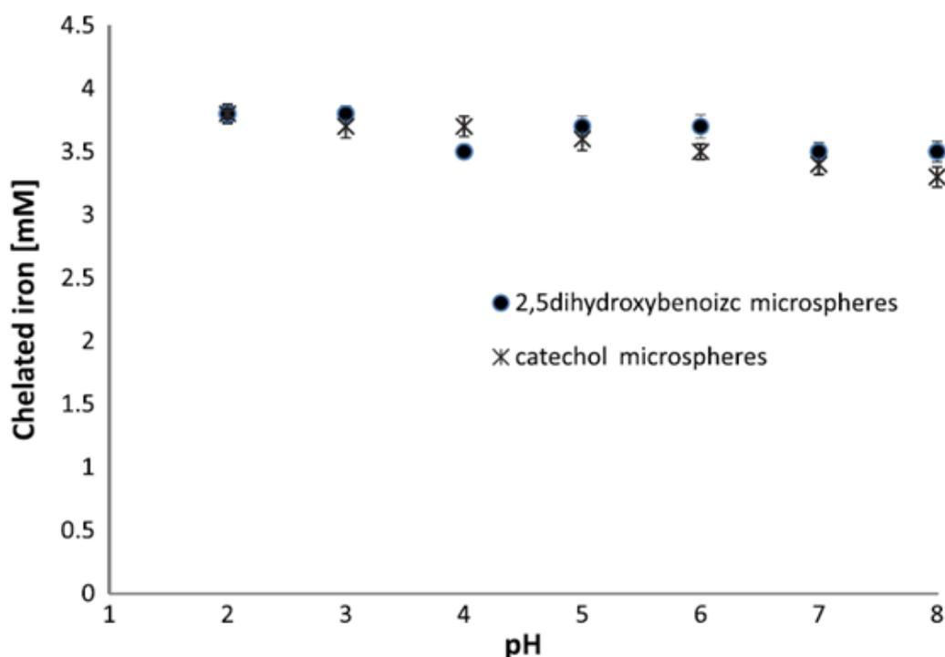
**Fig. 36.** Chelation of  $Fe^{2+}$  (3,8 mM initial concentration) by 2,5-dihydroxybenzoic acid and catechol functionalized microspheres
