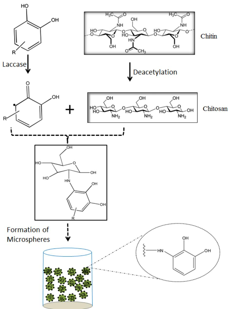
**Fig. 12.** Envisaged strategy for the enzymatic synthesis of catechol functionalized chitosan microspheres
