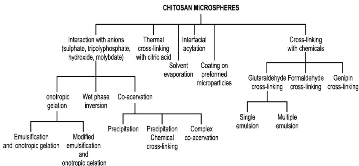
**Fig. 11.** Method for preparation chitosan microspheres (Sinha et al., 2004)
