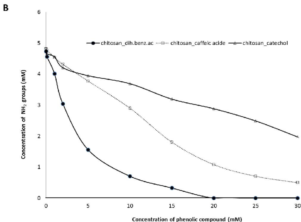
**Fig. 26B.** Consumption of  $-\text{NH}_2$  groups during enzymatic coupling of phenolic molecules to glucosamine and chitosan and the effect of the concentration of the phenolic molecules in coupling to 15 kDa chitosan
