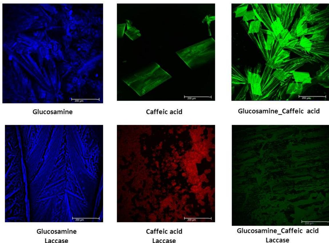
*Fig. 30. In vitro coupling reactions of caffeic acid molecules onto chitosan*
