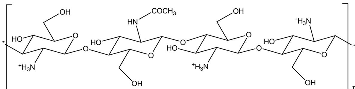
*Fig. 10. Molecular structure of chitosan*
