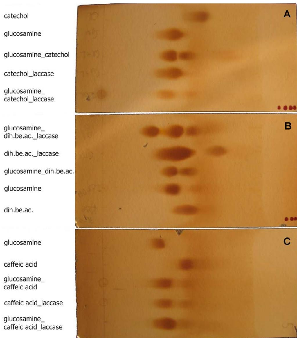
**Fig. 19.** (A) coupling reaction with catechol, (B) coupling reaction with dihydroxybenzoic acid, (C) coupling reaction with caffeic acid
