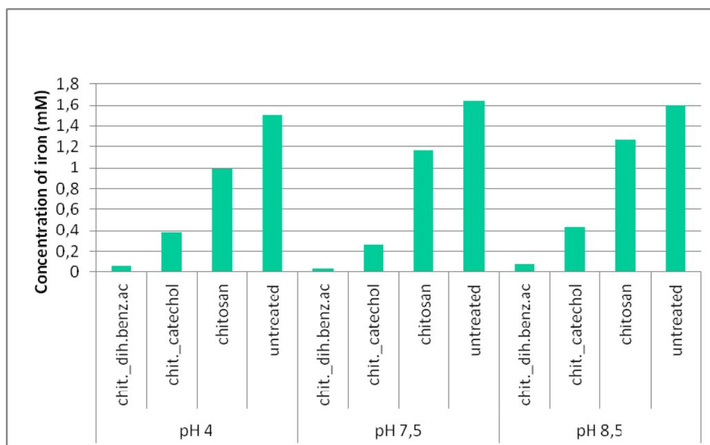
**Fig 39.** Iron binding capacity of catechol and dihydroxybenzoic acid functionalized microspheres
