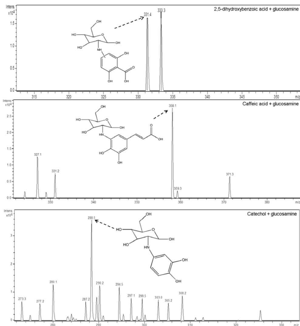
**Fig. 22.** HPLC-MS chromatograms of the laccase assisted coupling of 2,5-dihydroxybenzoic acid, caffeic acid, and catechol onto glucosamine
