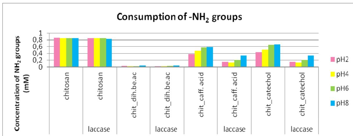
**Fig. 25.** Quantification of  $-\text{NH}_2$  groups on chitosan which determines the coupling efficiency depending on pH. Reaction with and without laccase
