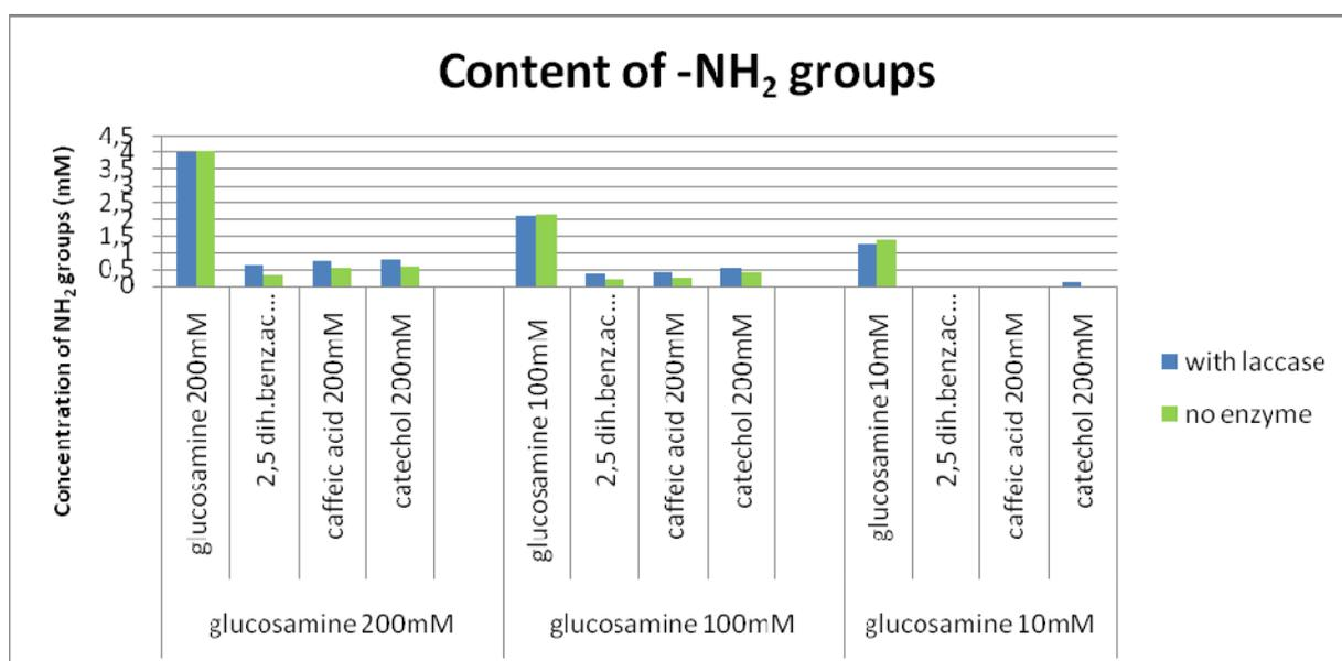
**Fig. 24.** Quantification of  $\text{-NH}_2$  groups on chitosan which determines the coupling efficiency depending on concentration of reactant
