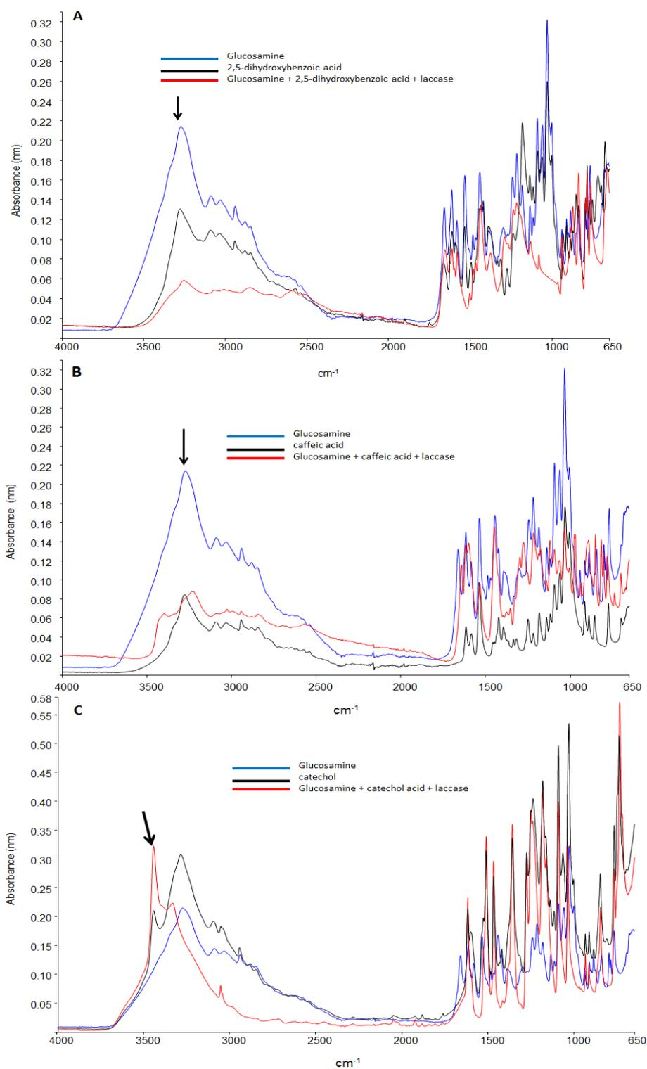
**Fig. 23.** FTIR spectra of different coupling of (A) 2,5-dihydroxybenzoic acid, (B) caffeic acid, and (C) catechol onto glucosamine
