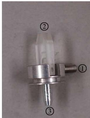
**Figure 25:** Typically used sample holder. (1): fixation screw, (2): sample, (3): fixation rod for ultramicrotomy & measurement.
