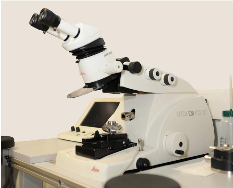
**Figure 22: The Ultramicrotome.**
