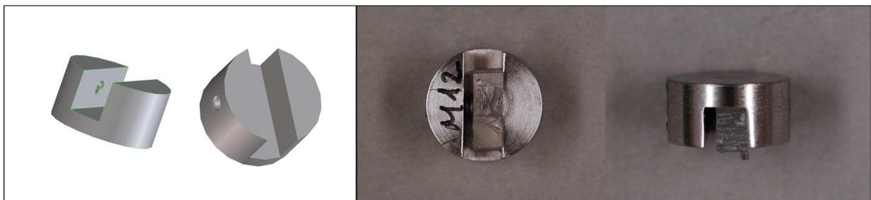
**Figure 26:** New sample holder. Left: 3D drawing of it. Right: Fabricated sample holder with sample
