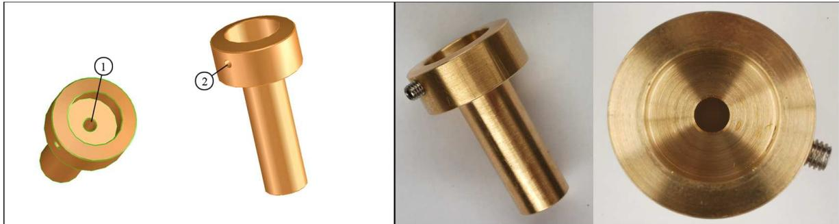
**Figure 27:** Fixation part for ultramicrotome use. Left: 3D drawing. (1) is the hole for stick holders, (2) is the drilling for the fixation screw. Right: after fabrication.
