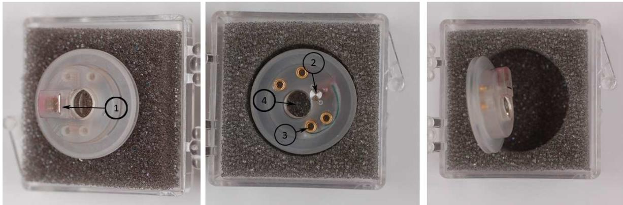
**Figure 46: The probe holder for liquid applications. (1) The fixation and trench for the probe. (2) Fixation spring. (3) Electronic circuit and fixation contacts. (4) Glass window for the optical laser. The shiny red rectangle is the build in piezo for cantilever oscillation.**
