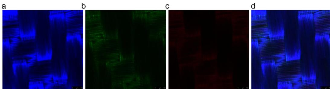
**Fig. 26: Sterile sample of textile examined with CLSM.** a) textile. b) green-fluorescent SYTO® 9. c) red-fluorescent propidium iodide. d) overlay. Scale bar: 100  $\mu\text{m}$ . For examination with CLSM, textile pieces were placed in a staining solution (LIVE/DEAD® Bacterial Viability Kit - BacLight™).
