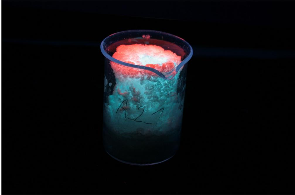
**Figure 4.18.:** Unsintered SA,Eu(1) under the UV lamp: the sample shows areas of green and red glowing, respectively. The chosen wavelength was 254 nm.
