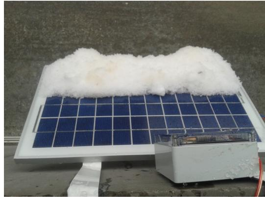
Figure 3.3: Not the entire snow layer slid off, however, due to the frame
