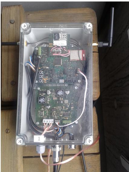
Figure 4.31: A sealed sensor node with harvesting system in case.
