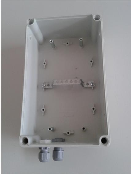
Figure 4.29: A barebone case with already drilled sensor connectors.
