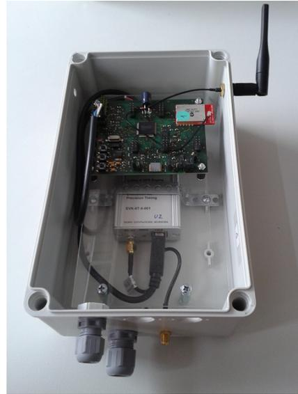
Figure 4.30: Including a GPS receiver and a sensor node mounted on plexiglass.
