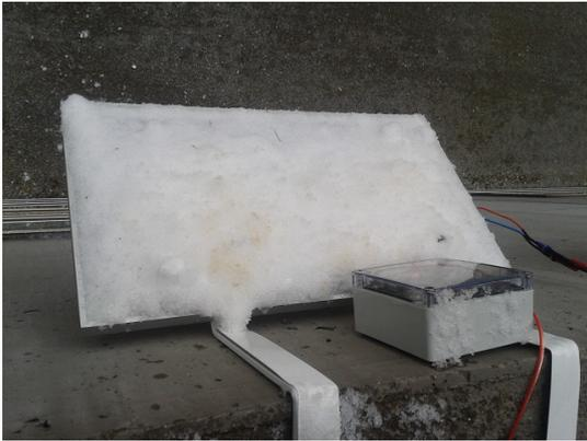
Figure 3.2: Solar cell covered in snow before reverse current mode
