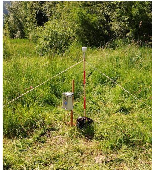
Figure 4.32: Complete system mounted on a rod with connected battery and GPS antenna. Test carried out in Wald am Schoberpass, Styria.
