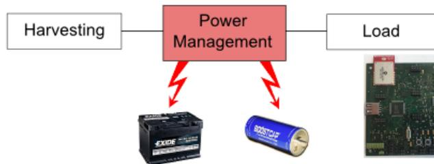
Figure 2.1: Architecture of an energy harvesting system. Power management will be the focus of this thesis.
