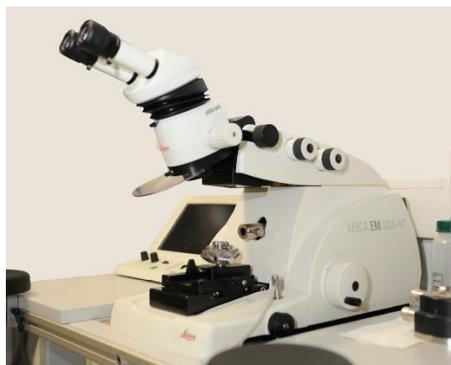
**Fig. 23:** Leica ultramicrotome. [32]
