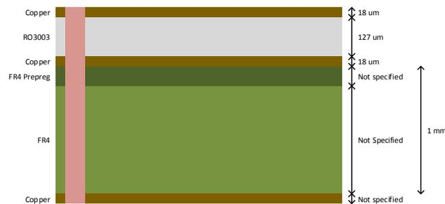
FIGURE 5.2: Stack-up of the AT&S Circuit Board
