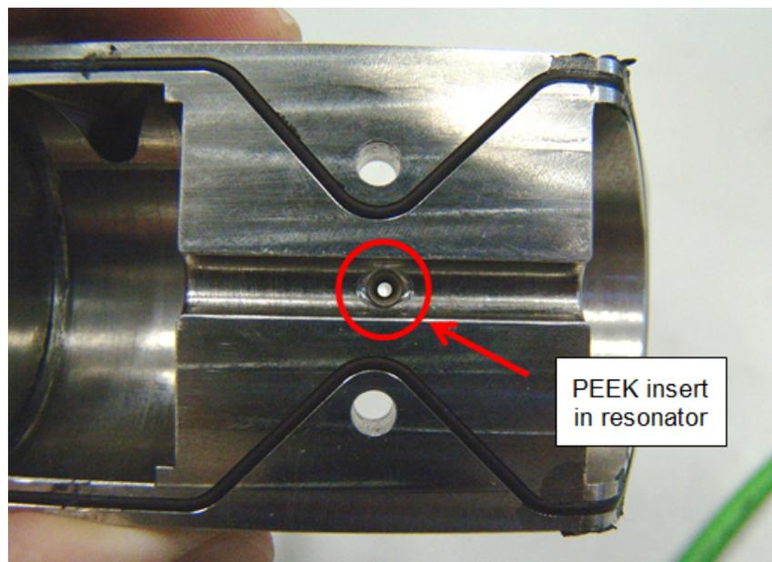
**Figure 30:** Polyetheretherketon PEEK insert to make the resonator diameter smaller from 3 mm to 1.5 mm
