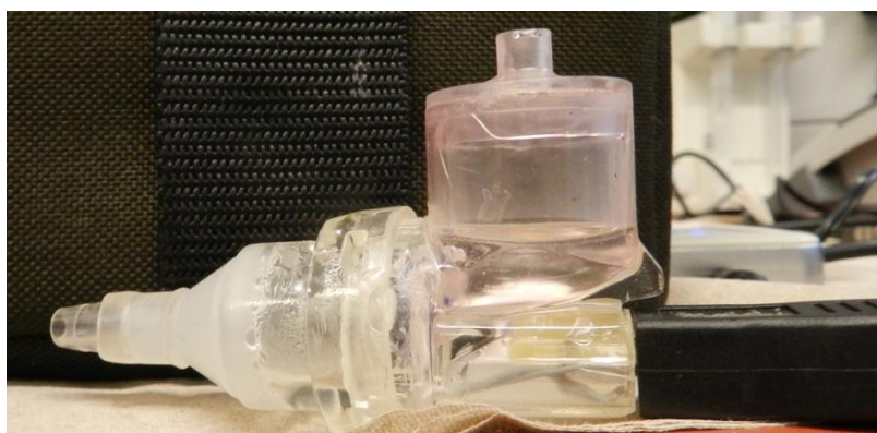
Figure 2. 2: M-neb mouse inhaler (NEBU-TEC) for IPL system
