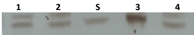
Figure 3. 33: LI-1 iloprost encapsulation efficiency after nebulization with MicroDrop® Pro, (1) aerosol liposomal iloprost EE ~50%, (2) aerosol free iloprost, (S) iloprost standard, (3) remainder liposomal iloprost EE ~70%, (4) remainder free iloprost. Aerosol and remainder samples contain in each case both bands together 4 µg of iloprost. The standard was 2 µg of iloprost.
