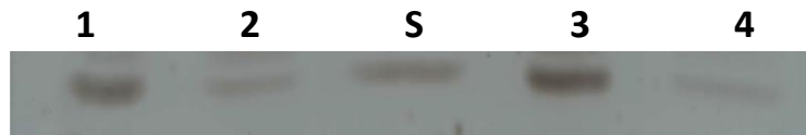
Figure 3. 40: LI-2 iloprost encapsulation efficiency after nebulization with eFlow® rapid, (1) aerosol liposomal iloprost EE ~80-90%, (2) aerosol free iloprost, (S) iloprost standard, (3) remainder liposomal iloprost EE ~80-90%, (4) remainder free iloprost. Aerosol and remainder samples contain in each case both bands together 4 µg of iloprost. The standard was 2 µg of iloprost.
