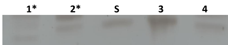
Figure 3. 36: LI-1 iloprost encapsulation efficiency after nebulization with Optineb®-ir, (1) aerosol liposomal iloprost EE ~20%, (2) aerosol free iloprost, (S) iloprost standard, (3) remainder liposomal iloprost EE ~80%, (4) remainder free iloprost. Aerosol and remainder samples contain in each case both bands together 4 µg of iloprost. The standard was 2 µg of iloprost. *The sample bands contain together only 1.7 µg iloprost due to insufficient sample volume.
