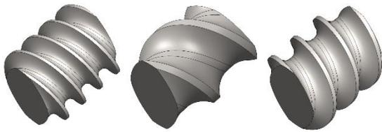
**Figure 11: Conveying elements with different pitch size, conveying direction (forward, forward, backward)**
