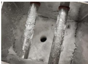
**Figure 49:** Cohesive powders tend to build bridges in the hopper, causing formation of an empty hole around the agitator
