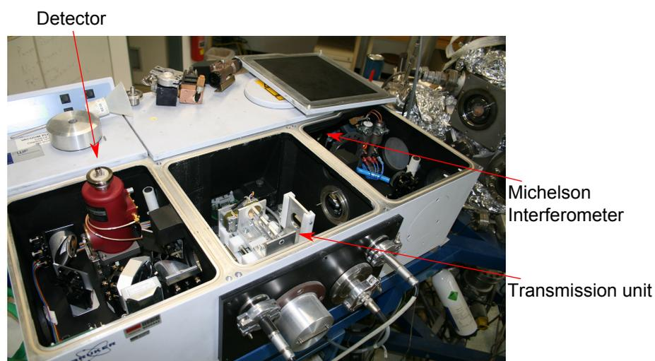
Figure 3.4: Bruker IFS 66 V Fourier transform infrared spectrometer.
