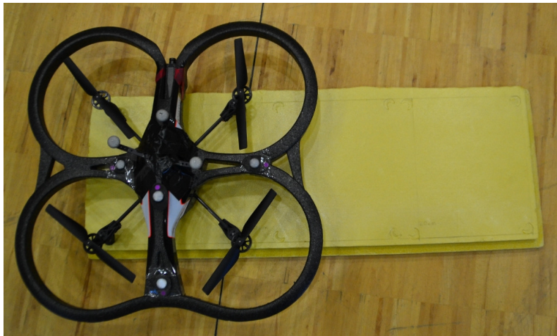
Figure 5.3: Parrot AR.Drone 2.0 with its protective indoor hull and seven reflective balls for tracking with the Vicon system.
