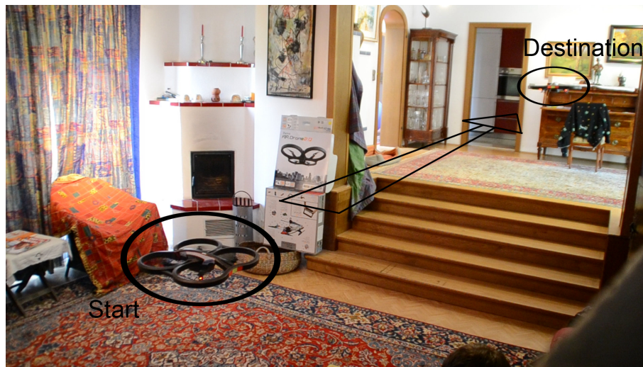
Figure 5.22: Mission for the multi level experiment. After initialization the MAV only has map points on the curtains. The mission is to safely move up the stairs and reach the destination facing the antique desk.
