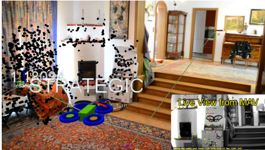
Figure 1.1: Active Visual Localization. Through the analysis of the sparse reconstruction (black dots) and actively exploring relevant parts of the scene, our system maintains the visual localization at all times during the way-point navigation.
