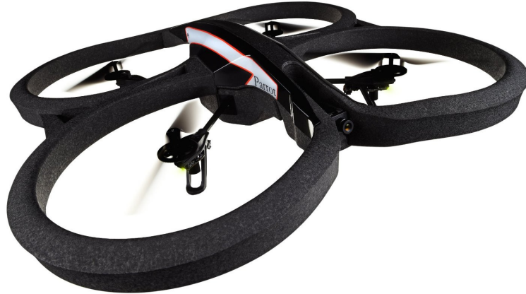
Figure 5.2: Parrot AR.Drone 2.0 with its protective indoor hull.
