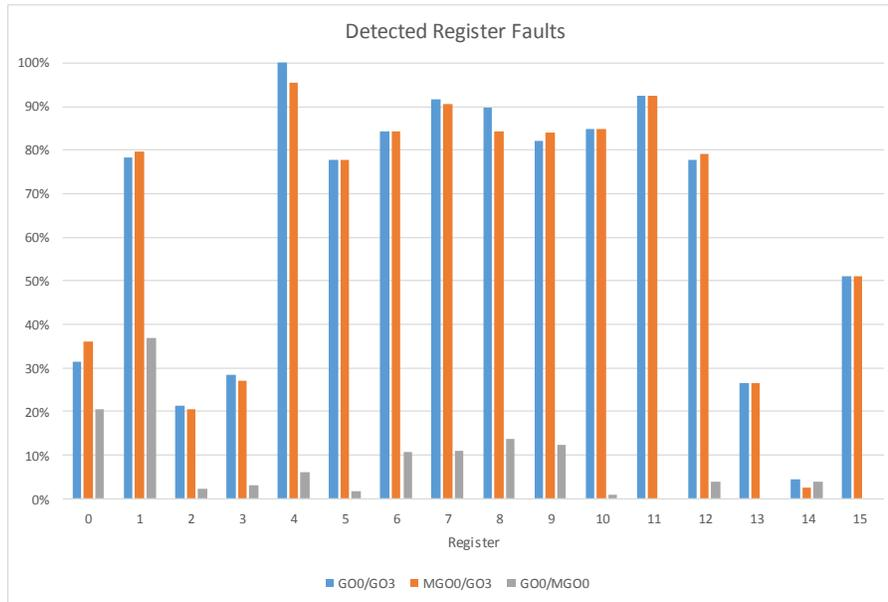
Figure 5.11: Source mutation: Detected register faults in percent for each register.
