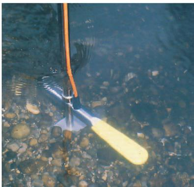
Abb. 16: Messinstrument [2] Nautilus C 2000
