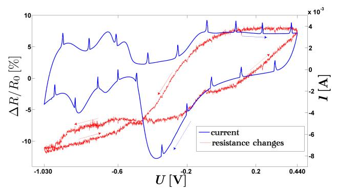
Figure 4.22:  $TUG-NCP_1$ ,  $R_0=0.00561~\Omega$ , resistance measurements during the  $3^{rd}$  cycle of a CV  $(U_l=-1030~{\rm mV}$  and  $U_h=440~{\rm mV},\,v=0.2~{\rm mVs}^{-1})$
