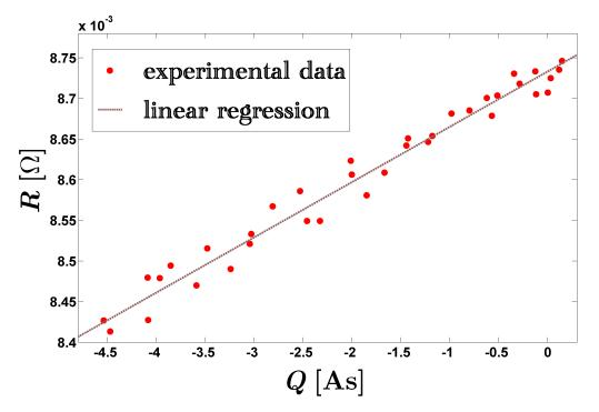
**Figure 4.25:** Sample  $TUG - NCP_2$ , further evaluation of figure 4.24, relating corrected resistance data with the recorded charge.
