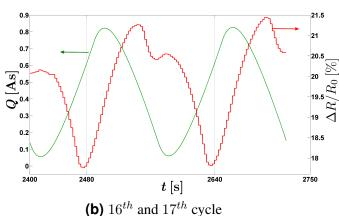
Figure 4.16: Sample  $TUG-NPP_5$ ,  $R_0=1.339~\Omega$ . Extract from the second CV, 20 cycles recorded with the same settings as before, see caption in figure 4.15a. The absolute changes in resistance reduced to  $\frac{\Delta R}{R_0} \approx 3\%$ . The complete plot is shown in the appendix figure B.1.
