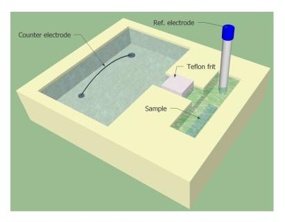
Figure 4.30: Draft of a possible experimental setup, designed for dealloying in an IL [58].
