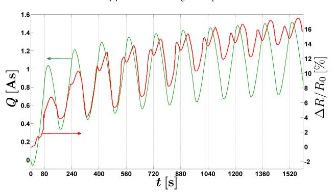
(b) Resistance and charging time dependence. The vertical lines mark the times at which the potential reached its maximum value ( $U_h = 400 \, \mathrm{mV}$ ).
