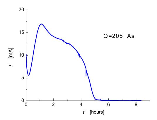
**Figure 4.4:**  $TUG-NPP_6$  dealloying current behaviour.  $U_{WE}=1.575\,\mathrm{mV}$  vs. 1-M Ag/AgCl in 0.5-M  $H_2SO_4$ .
