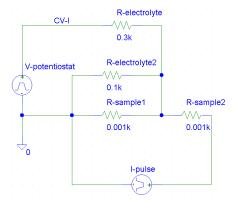
**(b)** Equivalent circuit for a potentiostat recording a voltammogram using two electrode geometry
