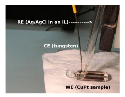
Figure 4.26: Experimental setup to dissolute Cu out of a  $Cu_{75}Pt_{25}$  starting alloy in an ionic liquid
