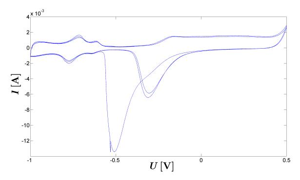
**Figure 4.6:** Cyclic voltammogram of a  $TUG - NPP_3$  sample fragment in 1-M KOH;  $v = 0.1 \,\mathrm{mVs^{-1}}$ , RE=saturated Ag/AgCl.
