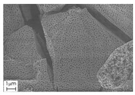
(b) SEM image of bicontinuous porosity created by the dealloying of  $Cu_{80}Pt_{20}$  in 1-M  $HClO_4$  at 1.24 V vs. NHE for 20 hours followed by heat-treatment at 800°C for 15 minutes (Reproduced by permission of The Electrochemical Society) [23].
