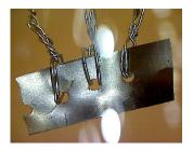
Figure 4.9: Sample cracked during the measurement
