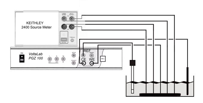
**Figure 3.4:** Experimental setup for resistance measurements
