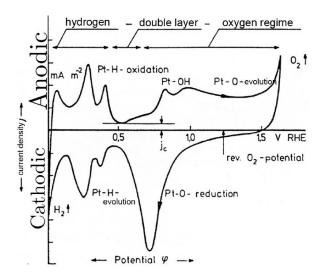
**Figure 2.1:** Schematic cyclic voltammogram of platinum, redrawn after [14]
