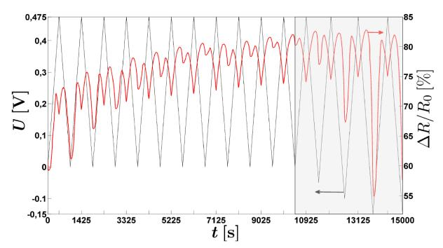
(a) Resistance and voltage time dependence. The marked section was used for the analyses shown in figure 4.17b.
