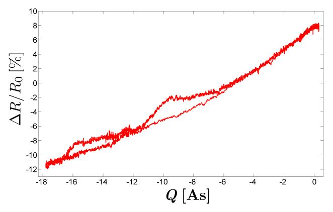
Figure 4.23:  $TUG - NCP_1$ , further analysis of figure 4.22. The slope in the regime assigned to oxide formation and its reduction  $(-10 \leftrightarrow 0 \text{ As})$  is  $\approx 1.4 \frac{\%}{As}$ .
