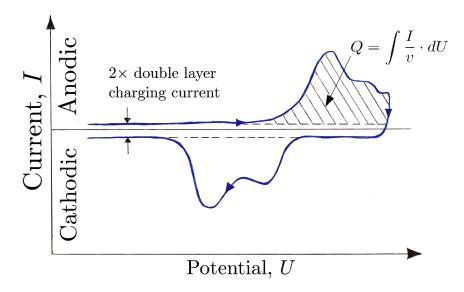
**Figure 2.3:** Typical cyclic voltammogram for an electrochemical surface process. The charge assigned to chemisorption only can be calculated from the shaded area.
