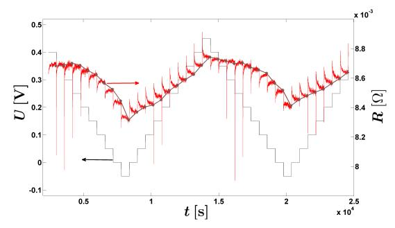
Figure 4.24: Sample  $TUG-NCP_2$ , time dependence of the resistance at different potentials successively applied with potential steps of  $50\,\mathrm{mV}$  after ten minutes. High currents perturb correct resistance measurements, which is apparent from the spikes in resistance observed at high current values after switching the voltage. The dark red dots mark resistance measurements at the end of each CA and should be regarded as the main result of this sequence.
