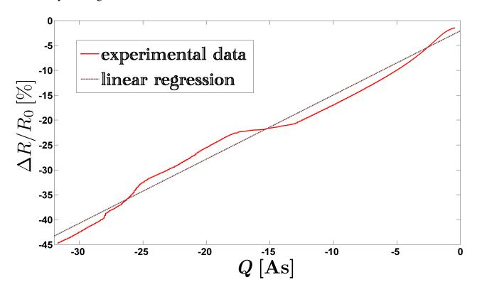
Figure 4.12: Sample  $TUG-NPP_2$ ,  $R_0=1.965~\Omega$ : Relation between charge and resistance during a CV, starting from  $U_{start}=300\,\mathrm{mV}$  reaching the potentials  $U_l=-586\,\mathrm{mV}$  and  $U_h=-486\,\mathrm{mV}$  for successive cycling  $(v=1\,\mathrm{mVs}^{-1})$ . The oxide layer is reduced during this sequence. The slope of the fit is  $\approx 1.287\,\frac{\%}{\mathrm{As}}$ .
