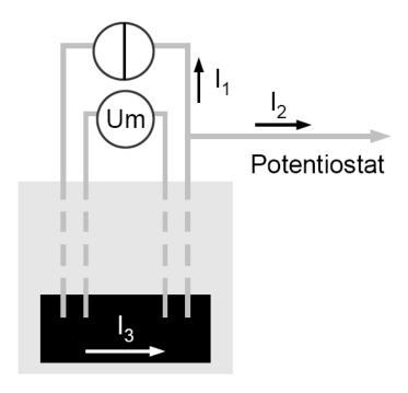
**Figure B.5:** Draft to explain the impact of currents into the potentiostat, on the resistance measurement
