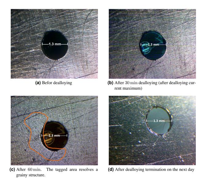
**Figure 4.5:** *In situ* microscopy during the dealloying process
