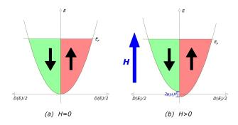
Figure A.1: Free electron model density of states D(E), without and with external magnetic field H [68]
