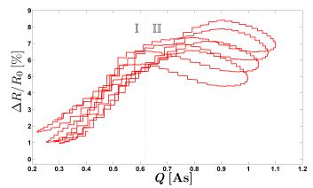
(b) Correlation of the resistance changes with the charge for the last four cycles of the first CV. The drift of the charge and resistance with time, was subtracted for this plot, using linear regression. The slope in section I is  $\approx 16.07 \, \frac{\%}{\text{As}}$ .
