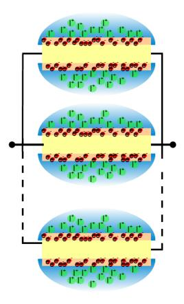
**Figure 2.9:** Draft of a parallel circuit comprising multiple "ligaments". The induced charge increases with the number of ligaments because of the larger surface area.
