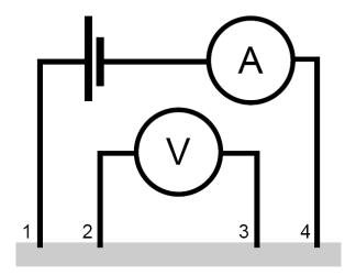
Figure 2.4: The basic idea of the four-point method
