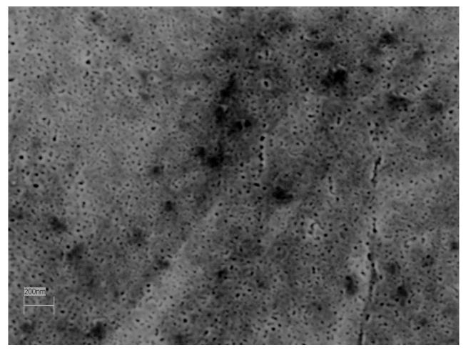
**Figure 4.1:** Sample  $TUG-NPP_2$  fragment, tempered twice at  $200\,^{\circ}\mathrm{C}$  for  $30\,\mathrm{min}$ . Nanoporosity is clearly visible.
