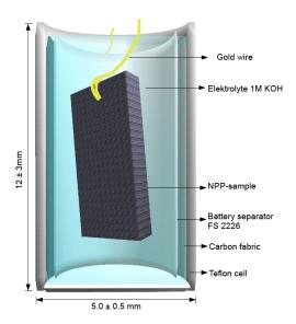
**Figure A.2:** Electrochemical cell with  $KIT - NPP_1$  as working electrode used for SQUID-measurements
