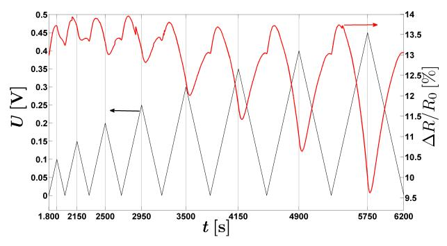
**Figure 4.20:**  $TUG-NPP_8,\ R_0=2.024\ \Omega.$  Sequence 12: CVs with increasing  $U_h$  values ( $U_{start}=U_h=0\,\mathrm{mV}\ v=1\,\mathrm{mVs}^{-1}$  and  $U_h=100,\ 150,\ 250,\ 300,\ 350,\ 400,\ 450\,\mathrm{mV}$ ). The vertical lines mark the times at which the potential reached its maximum value  $U_l$  to separate the cycles.
