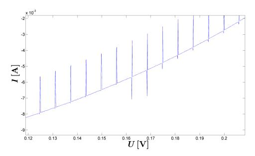
Figure 3.6: Additional peaks in a CV resulting from pulsed resistance masurements
