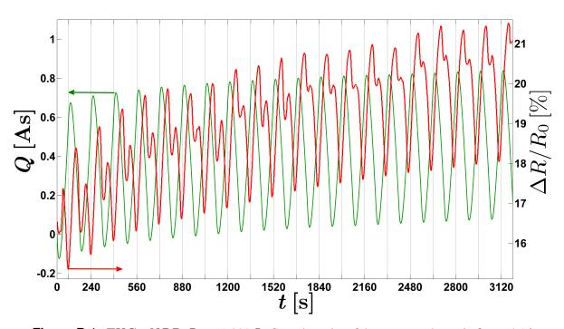
Figure B.1:  $TUG-NPP_5$   $R_0=1.339~\Omega$ . Complete plot of the excerpts shown in figure 4.16. Charge and resistance changes during the second CV recorded for this sample. The vertical lines mark the times at which the potential reached its maximum value  $Pot_h$ .
