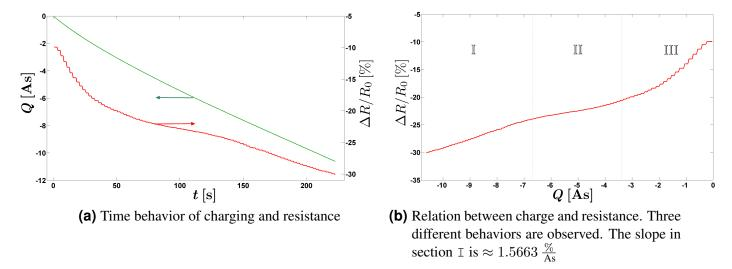
Figure 4.13: Sample  $TUG - NPP_3$ ,  $R_0 = 1.827 \Omega$ : CA at a potential of  $-586 \,\mathrm{mV}$ . At this potential reduction of the primary oxide layer occurs.
