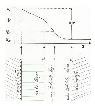
**Figure 2.2:** Draft of pseudo capacitive charging according to the Helmholtz model, and a schematic potential curve
