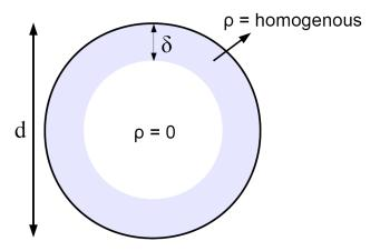
**Figure 5.1:** Principle of the *core-shell-model* described in [7]. Charging is assumed to affect only the charge density  $\rho$  in the outer shell.  $\rho$  remains constant inside the inner shell of  $(d - \delta)$  in diameter.
