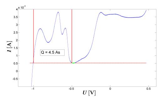
**Figure 4.8:** Determination of the charge, accociated with oxidation of deposited atomic hydrogen, out of an anodic sweep in a CV. The green data points were assigned to simple double layer charging and used to determine a regression to estimate and subtract double layer charging - red dotted line. Sample  $TUG-NCP_1,\,v=0.2\,\mathrm{mV},\,1\text{-M}$  KOH served as electrolyte and a saturated Ag/AgCl RE was used.
