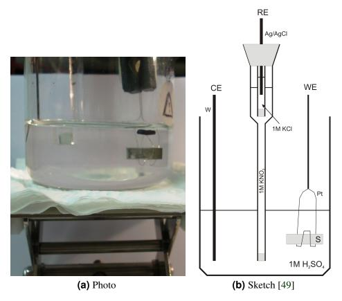
Figure 3.1: Set-up used for dealloying
