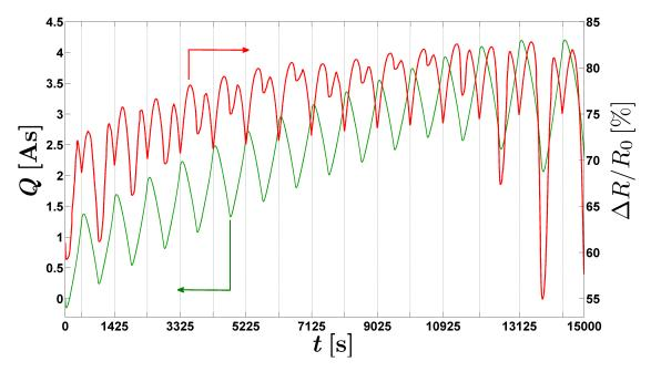
Figure B.2: Sample  $TUG-NPP_5$ ,  $R_0=1.339~\Omega$ . Additional plot for figure 4.17.Resistance and charge time dependence during a CV recorded (with decreasing  $Pot_l$  value for the last four cycles). The vertical lines mark the times at which the potential reached its maximum value  $Pot_h$ .
