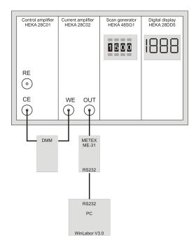
**Figure 3.2:** Equipment for recording currents and applying the desired potentials [49]
