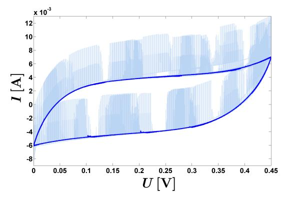
**Figure 4.19:**  $TUG - NPP_8$ , one of the first CVs,  $(U_{start} = U_l = 0 \, \text{mV})$  and  $U_h = 450 \, \text{mV}$ ,  $v = 1 \, \text{mVs}^{-1}$ ). The dark blue line designates the  $8^{th}$  cycle without the additional peaks resulting from the resistance measurement. Again, no peaks were observed that may explain the sign inversion of resistance changes.
