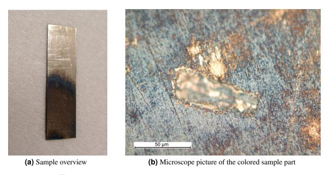
Figure 4.29: Sample after the aborted dealloying experiment in an IL
