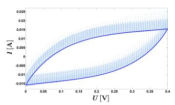
(a)  $CV(U_{start} = U_l = 0 \, \text{mV} \text{ and } U_h = 400 \, \text{mV}, \ v = 5 \, \text{mVs}^{-1}$ ). The dark blue line designates the  $7^{th}$  cycle without the additional peaks resulting from the resistance measurement, see chapter 3.4.1. No peak could be resolved, but integration of the CV lead to a positive total charge, green line in figure 4.14.
