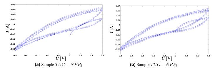
Figure 4.10: First CV of the samples  $TUG - NPP_{2-3}$ , both recorded using equal settings:  $U_{start} = 0 \text{ mV}, U_l = -500 \text{ mV}, U_h = 300, v = 5 \text{ mVs}^{-1}$ .
