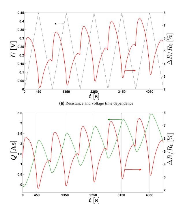
Figure 4.18:  $TUG-NPP_8$ ,  $R_0=2.024~\Omega$ . Charge and resistance behavior during one of the first CVs, details in the caption of figure 4.19. The vertical lines mark the times at which the potential reached its maximum value  $U_h$
