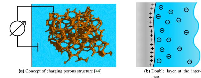
**Figure 2.7:** Principle of charge carrier depletion on the metal/electrolyte interface due to electrical double layer charging [12].
