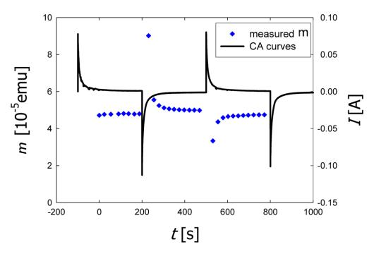
**Figure A.3:** Current influence on magnetic moment measurements (external field:  $H=500 \ Oe$ ).
