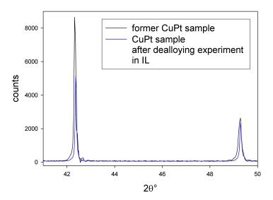
**Figure 4.28:** XRD analysis. Primary material versus the sample after the experiment: No change in the peak position and no peak broadening becomes obvious
