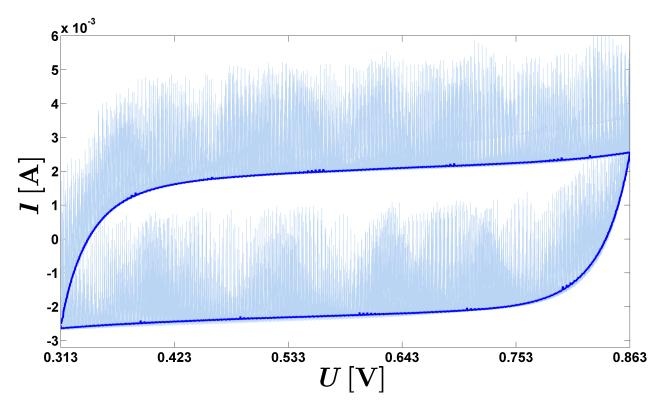
**Figure B.4:**  $TUG - NPP_8$  Complete CV of the sequence presented in figure 4.21a, and, figure B.3a. The dark blue line designates the  $8^{th}$  cycle without the additional peaks resulting from resistance measurements.
