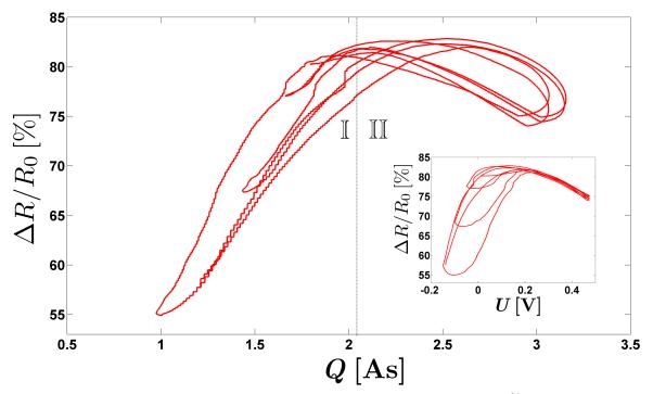
(b) Resistance dependence with charging. The slope in section I is  $\approx 15.12 \, \frac{\%}{\text{As}}$ . The linear correlation between the resistance and the potential in section II ( $\approx 0.20 - 0.45 \, \text{V}$ ) becomes obvious from the insert.
