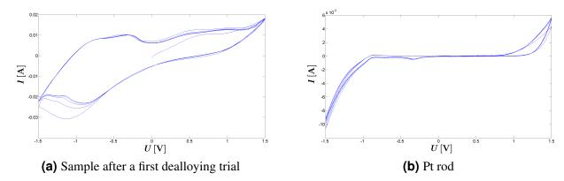
**Figure 3.3:** CVs of different platinum samples recorded with the same settings:  $U_l = -1500 \,\mathrm{mV}$ ,  $U_h = 1500 \,\mathrm{mV}$ ,  $v = 100 \,\mathrm{mVs^{-1}}$ . Because of extremely high overpotentials for the porous sample, no hydrogen or oxygen evolution was observed at such extreme  $U_l - U_h$  values, in contrast to the planar platinum rod (1-M KOH electrolyte, potentials measured vs. saturated Ag/AgCl)
