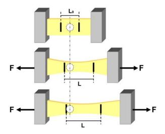
Figure 5.2: Problems with inhomogeneities in the sample on unidirectional stretch. In this example the left clamp is fixed and only the right clamp moves. As the position of the X-ray beam (indicated by the dashed circle) stays constant, the part of the tissue viewed by the beam changes. In the case of an inhomogeneous composition of the tissue this will cause inconsistent signals in the diffracted images.
