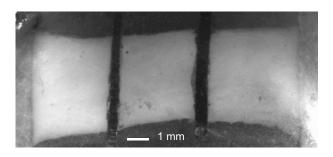
Figure 5.5: A sample as viewed by the video-extensometer. The black vertical lines are the markers that are used for length measurements. The load axis is in the horizontal direction in the image.
