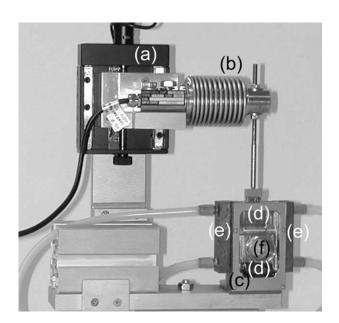
Figure 4.3: Tension cell: the sample is mounted between two clamps (d), of which the upper one is moved by a translation stage (a). Force is measured using a load cell (b), on which the upper clamp is mounted.
