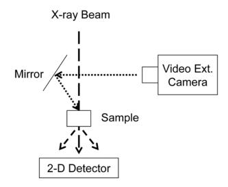
Figure 4.4: Schematic drawing of the set-up as installed in the beamline.
