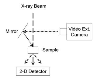
Figure 5.4: Schematic drawing (top-view) of the setup as installed in the beamline. A mirror reflects the image of the sample to the video camera. The angle between the mirror and the X-ray beam equals almost 45ř, hence distortion of the image is negligible. Moreover the camera is calibrated to each sample.
