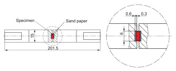
Figure 7.4: Schematic direct tension fixing tool with a detailed drawing of the specimen-rod connection. Dimensions are given in mm.
