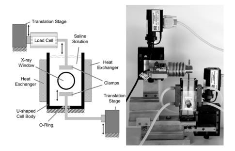
Figure 5.3: Tension cell: the sample is mounted between the two clamps, which can both be moved by PC controlled translation stages. Force is measured by a load cell mounted on the upper translation stage. Heat exchangers on either side of the cell allow to maintain a constant temperature of the tissue bath. X-rays pass through two X-ray windows.
