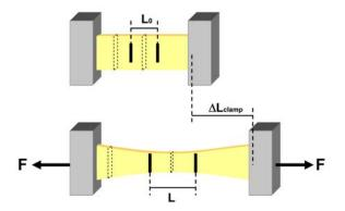
Figure 5.1: A soft tissue sample in unloaded state and stretched with the force F. The sample is mounted between two clamps. The nonlinear shrinkage of the sample width is illustrated. The central part — defined by two markers — of a sufficiently long sample can be considered as roughly cuboid. The distance of the markers allows the reconstruction of the cross sectional area and hence the calculation of the true stress.
