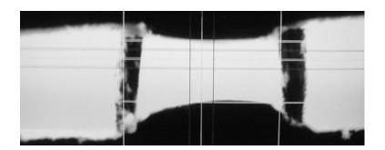
Figure 4.2: Stretching of a representative sample as viewed by the videoextensometer. The black vertical lines are the markers for length measurements (length is in the horizontal direction in the image).
