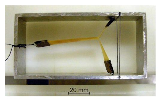
Figure 7.7: Photograph of a mechanically fixed specimen in the specimen holder.
