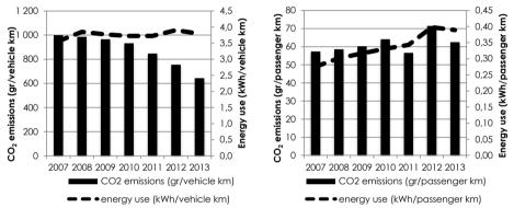
Figure 3: CO<sub>2</sub> emissions and energy use per vehicle kilometer and per passenger kilometer (national level, from 2007 to 2013) (Svensk Kollektivtrafik, 2014a; Trafikanalys, 2015-personal communication)
