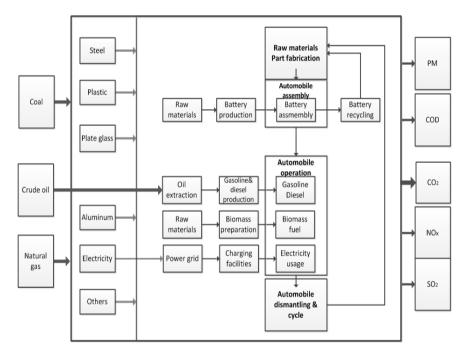
Figure 7: Life cycle of a vehicle
