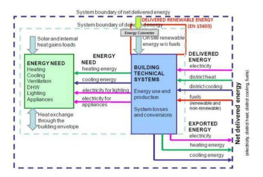
Note. The box of "Energy need" refers to rooms in a building and both system boundary lines may be interpreted as the building site boundary. Source [REHVA 2012].
