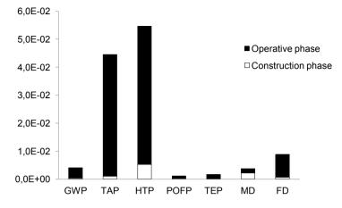
Figure 4.1 Normalized impacts calculated for construction and operative phases of the MARSS plant (attributional approach, referred to a functional unit of 1 kWh of exergy delivered).
