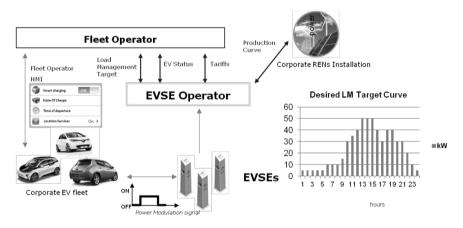
Fig. 5. Architecture of Electric Mobility Management system developed by Enel Group
