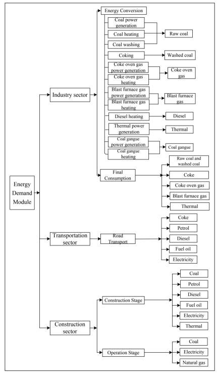
Figure 6: The overall structure of the LEAP-Handan model
